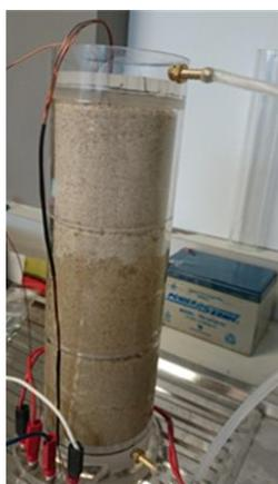
Fig 1: Schematic drawing of the experimental set up (flow cell)
