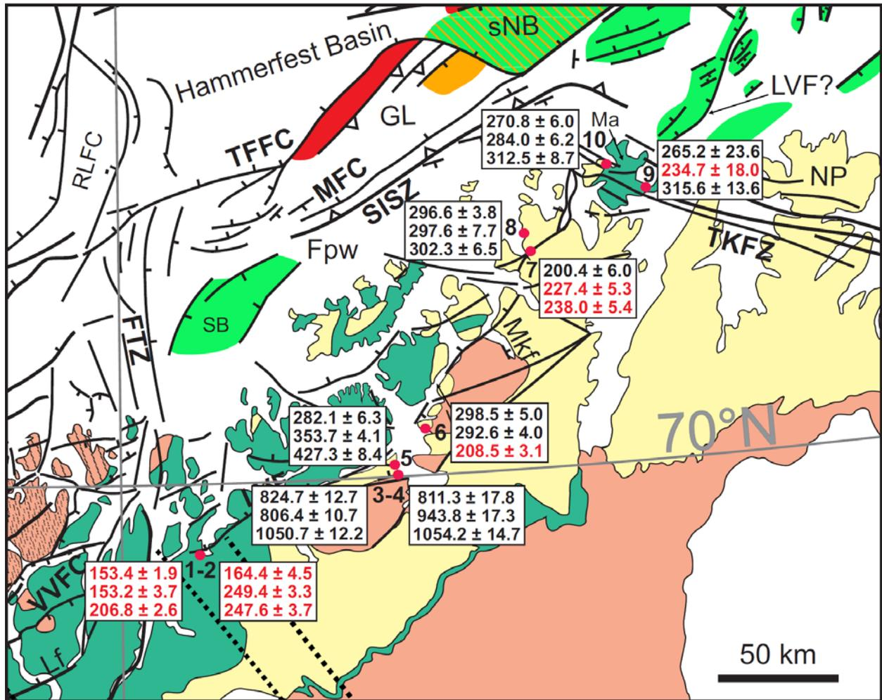
Figure 4: Structural map of the study area showing the obtained K–Ar ages for each sample in Ma, including from top to bottom finest, intermediate and coarsest grainsize fraction ages. Ages in red are considered erroneous (see main text). Map modified after Indrevær et al., (2013) and Koehl et al. (2018). Legend and abbreviations as in Figure 1.
