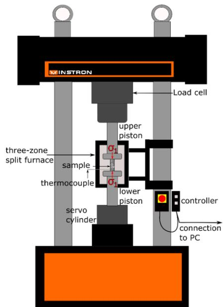
Figure 2. Schematic of the uniaxial compressive strength testing set-up in the Experimental Volcanology and Geothermal Research Laboratory at the University of Liverpool. A 100 kN Instron 8862 uniaxial press with a three-zone, split cylinder furnace was used to perform experiments at varying strain rates and temperatures.
