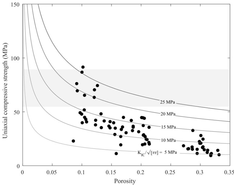
Figure 11 Plot of uniaxial compressive stress against porosity showing the ambient temperature mechanical data (black dots), alongside contours of various values of  $\frac{K_{IC}}{\sqrt{\pi r}}$  (5–25 MPa) from the pore-emanating crack model (Eq. 2). The range of UCS given by the
