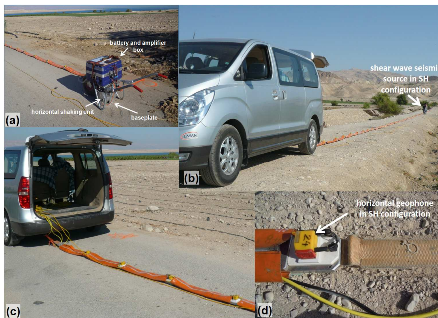
Figure 3: Photos of the shear wave seismic reflection acquisition campaign carried out in October 2013. (a) Wheelbarrow-mounted shear wave source system on asphalt pavement at start location of profile 2. (b) Recording car, towed land streamer and source during operation on profile 3. (c) Land streamer towed by the recording car during acquisition on profile 2. Colour paintings on the road surface were used for location numbering along the profiles. (d) Sledge-mounted horizontal geophone in SH (particle movement perpendicular to profiling direction) configuration along profile 3.
