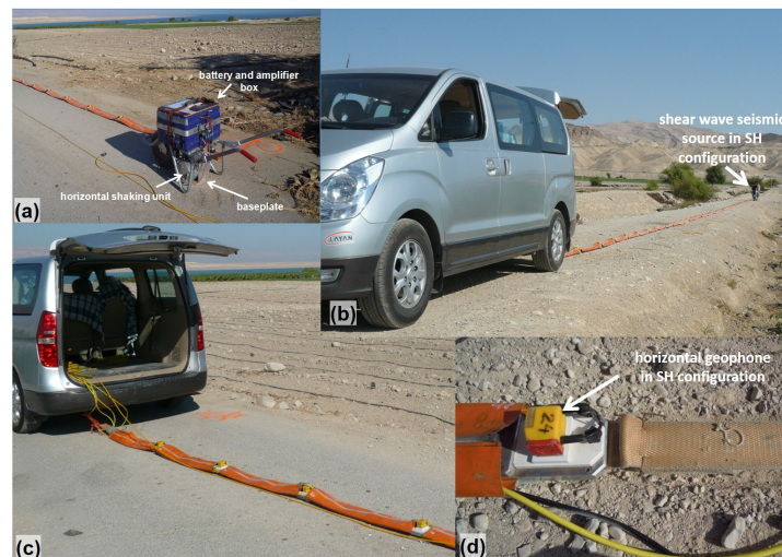
Figure 3: Photos of the shear wave seismic reflection acquisition campaign carried out in October 2013.
