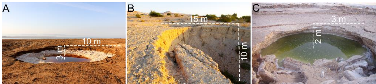
Figure 2: Sinkhole examples from the eastern shoreline of the Dead Sea. (A) Sinkhole with depth/diameter ( D_e/D_i ) ratio \sim 0.15 formed in semi-consolidated lime-carbonate mud of the former Dead Sea bed. (B) Sinkhole with D_e/D_i \sim 0.33 , formed in semi-consolidated sandy-gravel (alluvial) sediment. Note the deep cracks and tilted blocks marginal to the sinkhole. (C) Sinkhole with D_e/D_i \sim 0.33 formed in semi- to well-consolidated salt material. Note the typical overhanging sides and pronounced cracks in the surroundings.
