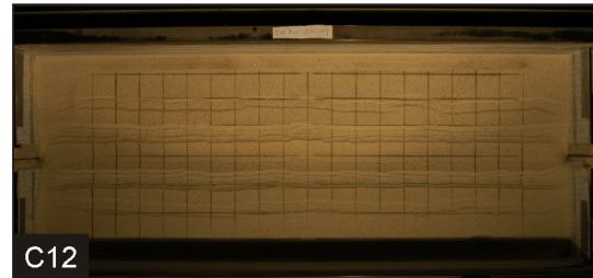
Fig. B2. Reproducibility tests. Final top views of experiments P2, C2 and C3 (brittle-only asymmetric plate base [P] and conveyor base [C]), C9-C11 (brittle-viscous conveyor base models, 4:1 brittle-viscous thickness ratio, high velocity: 40 mm/h [C10/C11] and 80 mm/h [C9]) and experiments P9 and C12 (brittle-viscous plate base [P] and conveyor base [C], half layer thickness, high extension velocity: 80 mm/h).
