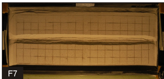
Fig. B1. Reproducibility tests. Final top views of experiments F2-F4 (brittle-only, foam base, with seed), F6 and F7 (brittle-viscous foam base, with seed), P6 and P7 (brittle-viscous plate base models, no seed) and C4-C6 (brittle-viscous conveyor base, no seed). Note that C5* and C6** were attempts to decrease boundary effects by replacing part of the basal viscous layer with sand (transparent overlay) or adding a lubricant (hand soap) along the short ends of the set-up, respectively. The former however increased boundary effects, whereas the latter did not significantly change surface structures and was therefore halted after 2 hours. Extension velocities are 8 mm/h in all cases.
