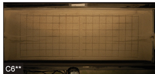
Fig. B1. Reproducibility tests. Final top views of experiments F2-F4 (brittle-only, foam base, with seed), F6 and F7 (brittle-viscous foam base, with seed), P6 and P7 (brittle-viscous plate base models, no seed) and C4-C6 (brittle-viscous conveyor base, no seed). Note that C5* and C6** were attempts to decrease boundary effects by replacing part of the basal viscous layer with sand (transparent overlay) or adding a lubricant (hand soap) along the short ends of the set-up, respectively. The former however increased boundary effects, whereas the latter did not significantly change surface structures and was therefore halted after 2 hours. Extension velocities are 8 mm/h in all cases.
