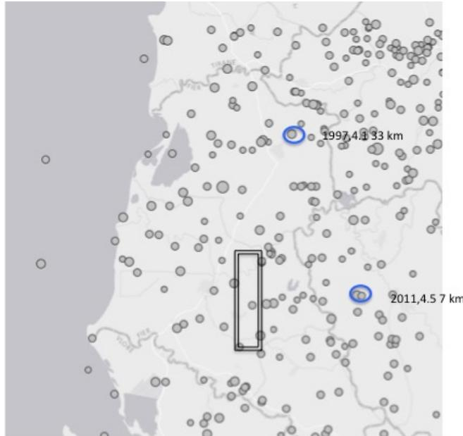
**Fig. 2.** Figure R2: Seismicity map around the Patos-Marinza oil fields.  $M \geq 2.5$  earthquake, 1973-2019, from USGS catalogue. Black box is the schematic contour of the Patos and Mazrinza oil-fields.
