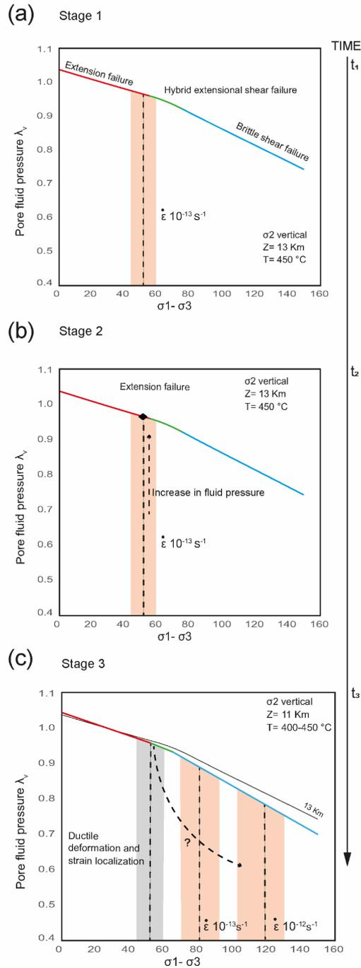
775 **Figure 13.** Conceptual model of the temporal and mechanical evolution of the BFZ045 fault zone (see text for more details). BFZ045 was characterized by (a) the development of mylonite creeping at ca.  $10^{-13} \text{ s}^{-1}$ , followed by (b) a transient increase in fluid pressure responsible for the emplacement of quartz veins. Ductile deformation then continued under increasing differential stress and strain rates (c).
