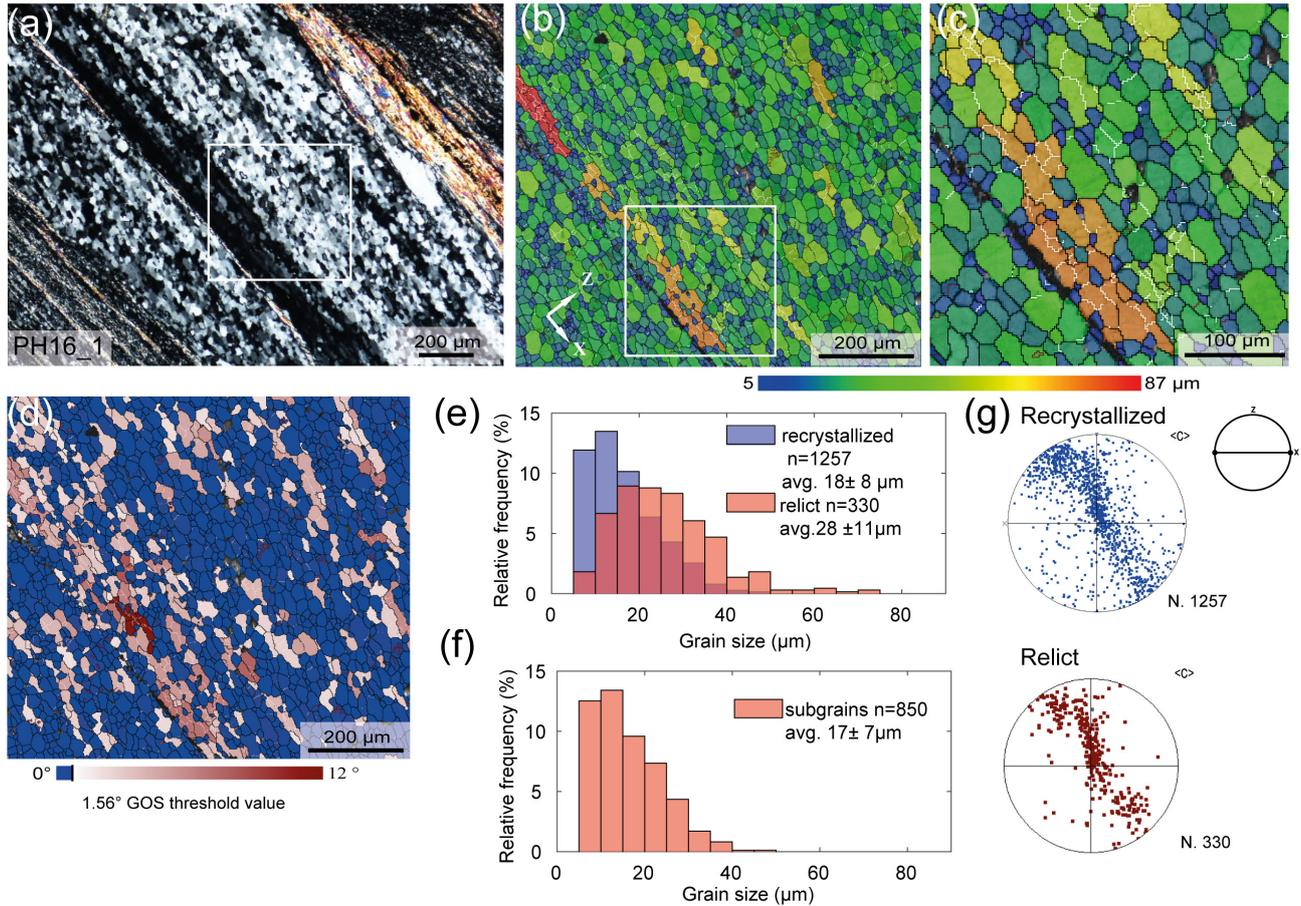
725 Figure 7. EBSD data of quartz from a recrystallized ribbon in the mylonite. (a) Polycrystalline ribbons of recrystallized quartz
