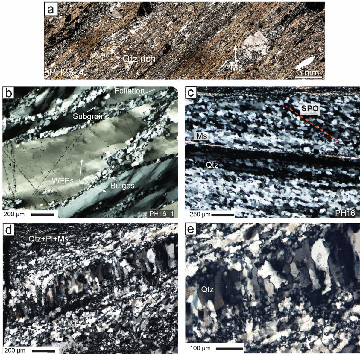
690 Figure 4. Microstructure of the BFZ045 mylonite. Cross-polarized light. (a) The mylonitic foliation is defined by the alternation of
