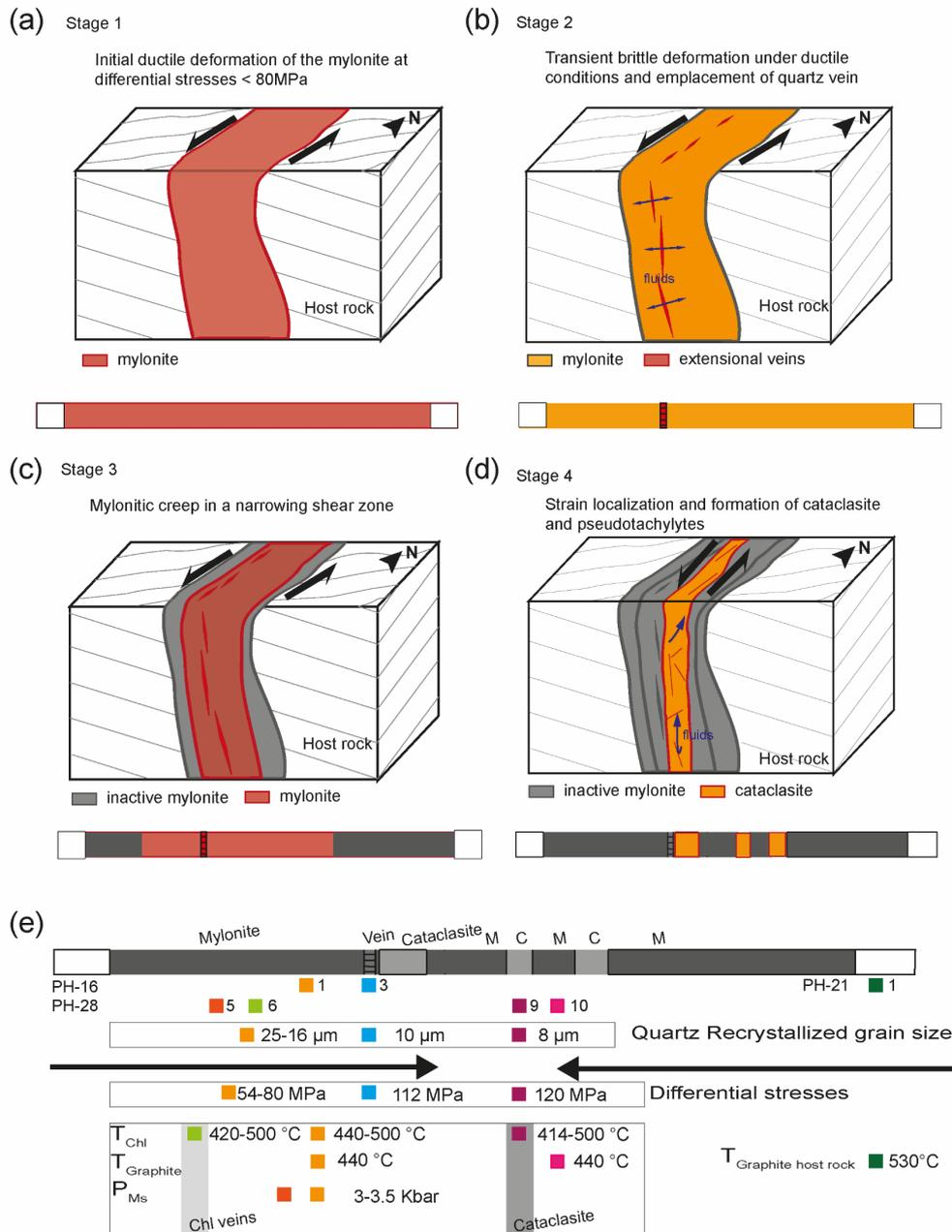
765 **Figure 12. Schematic representation of the microstructural evolution of BFZ045. (a-d) Grey lines: traces of metamorphic foliation in the host rock. In the schematic fault scheme evolution, red displays the active deformation process, grey represents the inactive deformation processes, and orange suggests a transition in the deformation. (a) The development of mylonite was punctuated by the emplace-**
