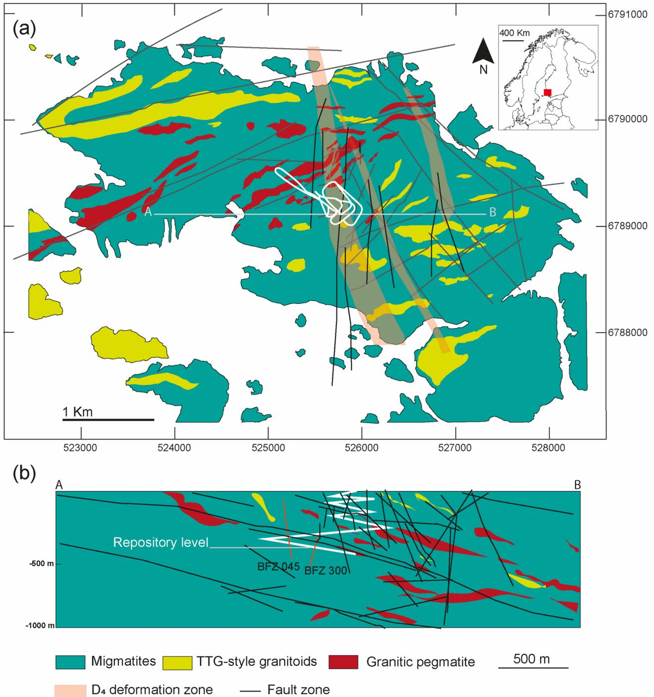
665 **Figure 1. Geological setting of Olkiluoto, SW Finland (inset on top-right). (a) Schematic geological and structural map, showing surface intersection of modelled brittle fault zone (BFZ) and ductile deformation zone, modified from Aaltonen et al. (2016) and Skytta and Torvela (2018). Coordinates for zone 34N in UTM coordinate system. The white line indicates the location of the**
