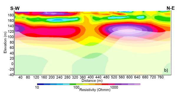
560 Figure 4. Results of the ERT performed preliminarily to the drilling of the DWVP 01 well (the location of the midpoint of the line is shown in Fig.1a, highlighted by a yellow circle). The sensitivity of the data with respect to the model parameter values reduces significantly below the depth of investigation (DOI – Asch et al., 2015) that is indicated by the white overlay.
