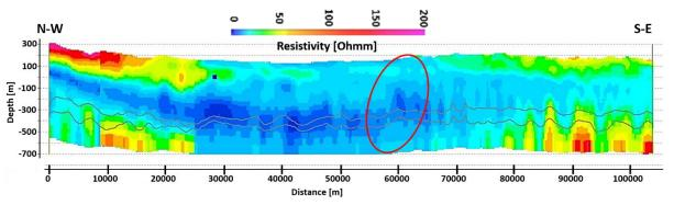
625 Figure 8. Cross-section along NW-SE line 7 (Fig. 1a) showing faulting (within the red circle) in the Bimbila. The DOI is showed as a solid grey line (there are two of them accordingly to their definition – more details on this distinction can be found in Christiansen and Auken, 2012).
