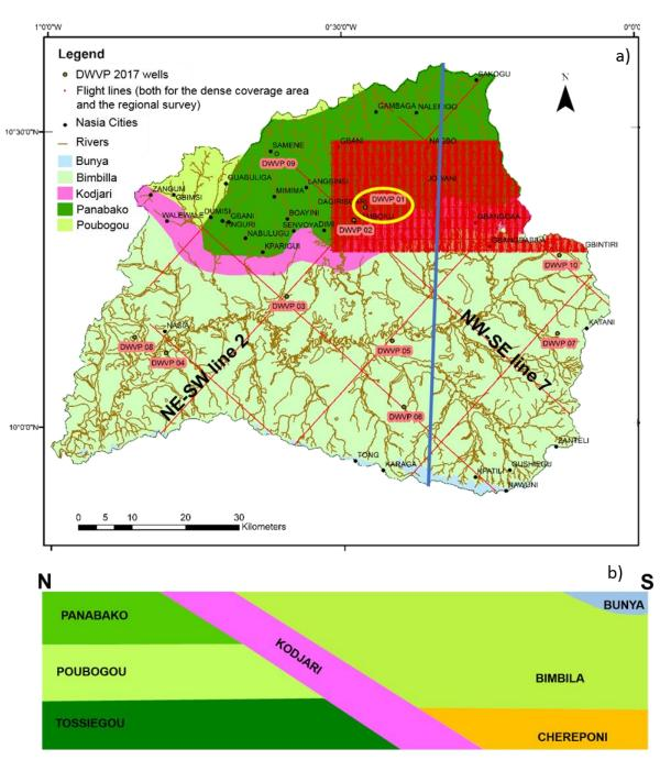
550 Figure 1: (a) Geologic Map of Nasia sub-basin after Carney et. al (2010); (b) Conceptual Model of the geology along a cross sectional N-S line within the study area (solid blue line in the panel a).
