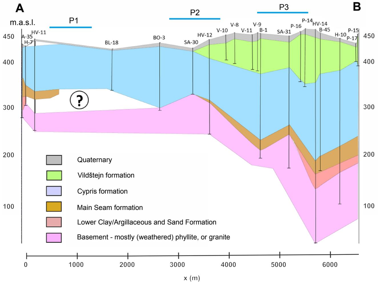
**Figure 3.** [Lithological transect along the large-scale profile, based on the descriptions of boreholes from the Czech Geological Survey \(former GEOFOND\). Question mark indicates an area of unknown lithology and the uncertainty of whether Main Seam and Lower Clay \(or Argillaceous-\) Sand formation are present in this area. P1 - P3 mark the locations of the small-scale ERT profiles. For each drill's location, please refer to Fig. 2.](#)
