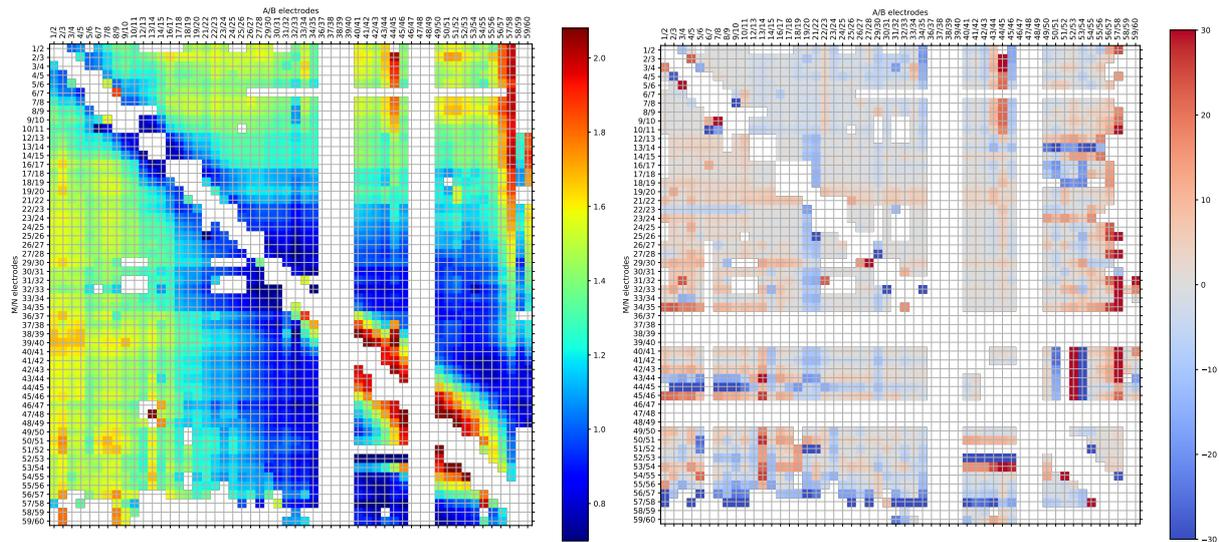
**Figure 5.** Full Raw data. Left: Apparent resistivity ( $\log \rho_a [\Omega m]$ ) all retrieved AB-MN pairs) as a function of current A/B-AB and potential M/N-MN dipoles. Left: Apparent resistivity ( $\log \rho_a [\Omega m]$ ), Right: Reciprocity Relative reciprocal error between forward (starting with current dipole 1/2) and reverse measurements (%).
