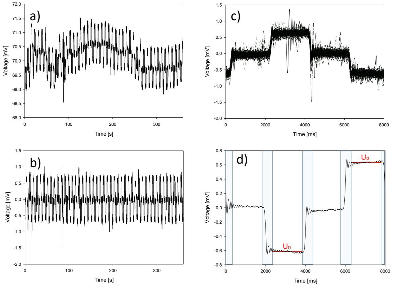
**Figure 4.** Processing steps of time series on an example. a) Raw time series  $U(t)$ , b) Time series  $U_{dr}(t)$  after drift correction, c) Stack distribution after cross-correlation, d) Mean stacked signal with rejection windows to delete current switch effects (greyish areas) with positive ( $U_p$ ) and negative ( $U_n$ ) mean plateaus.
