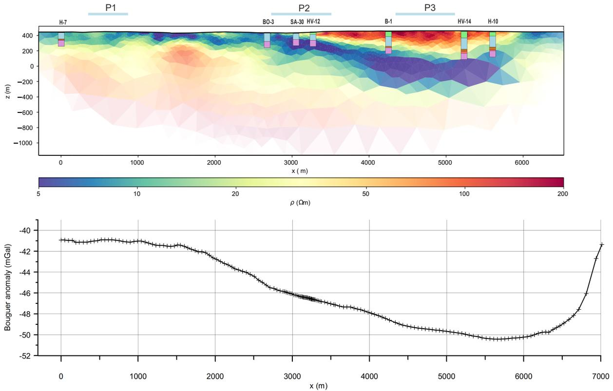
**Figure 8.** Inversion result (resistivity distribution) of the large-scale profile with the lithology columns of the boreholes (top) and the Bouguer gravity (bottom). *z: m.a.s.l.*. Colors for each stratigraphic unit is identical to Fig. 3: green - Vildštejn formation, lightblue-light-blue - Cypris formation, brown - coal, red - basal clay Lower Sand formation, pink - phyllitic/granitic basement.
