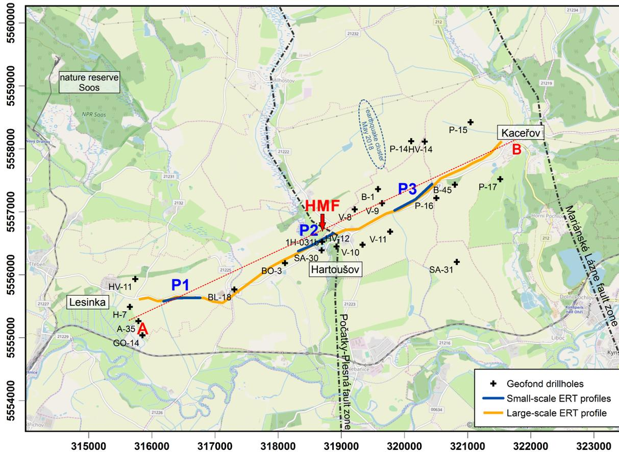
**Figure 2.** Map of the measured large-scale ERT profile (6,5 km), small-scale 625-700 m long ERT profiles (P1, P2, P3), and existing drill holes (Czech Geological Survey) with lithological information. Red dotted line marks the location of the lithological transect in Fig. 3. The Počátky-Plesná zone (PPZ) and Mariánské Lázně fault zone (MLF) are drawn as the main tectonic features. HMF = Hartoušov mofette field.
