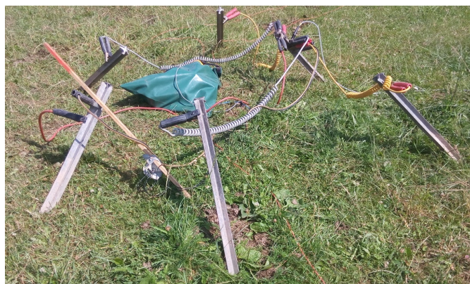
Figure 4. Current injection spot and a potential electrode with data logger protected by weather-proof bag. A minimum of six steel rods need to be driven into ground to guarantee proper current injection.
