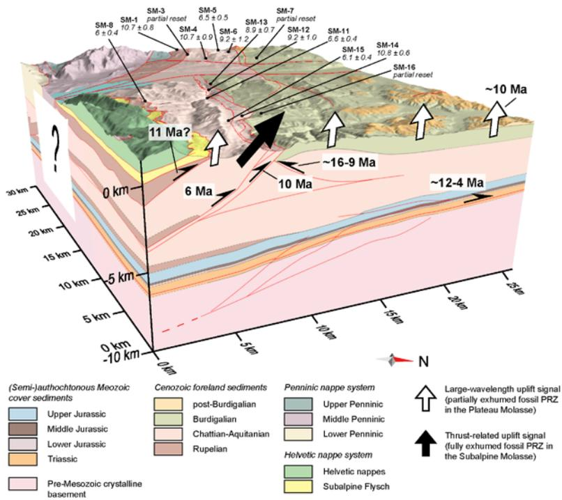
**Figure 4.** Block model of with sample locations and corresponding average (U-Th-Sm)/He ages. The construction of the block model is based on surface (Beck, 1945; Haus, 1937; Jordi, 2012; Rutsch, 1947; Schlunegger et al., 1993, 1997) and subsurface (2D seismic interpretation; Mock and Herwegh, 2017) geological information. PRZ, partial retention zone.
