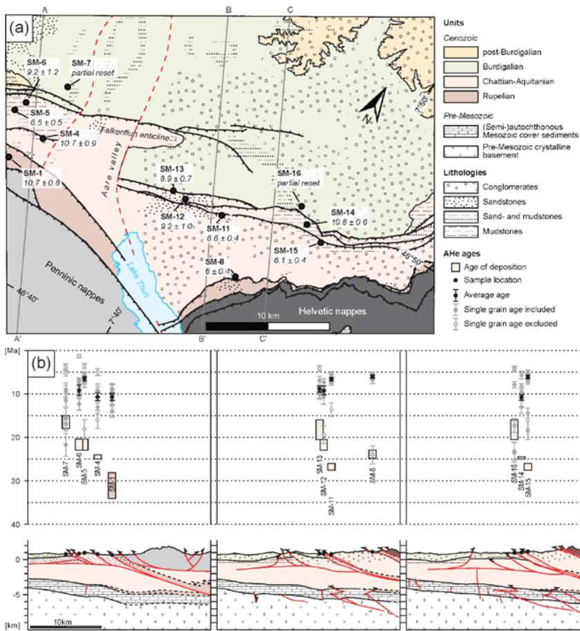
**Figure 2.** (a) Litho-tectonic map of the Lake Thun area showing sample locations and corresponding average apatite (U-Th-Sm)/He (AHe) ages. Traces of cross-sections A-A', B-B', and C-C' in Fig. 2b are given as black lines. The location of the sampling area is shown as a dashed rectangle in Fig. 1a. Note the arrow indicating north. (b) Cross-sections through the sampling area west (A-A') and east of the Aare valley (B-B' and C-C'), showing single grain and average AHe ages.
