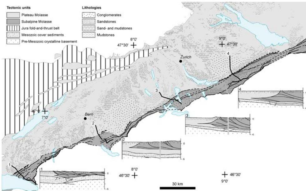
**Figure 6.** Litho-tectonic map of the Swiss Molasse Basin (modified from Landesgeologie, 2005). Cross-sections 1-4 are based on 2D seismic interpretation (cross-section 2, Mock and Herwegh, 2017; cross-sections 1, 3, and 4, Sommaruga et al., 2012).
