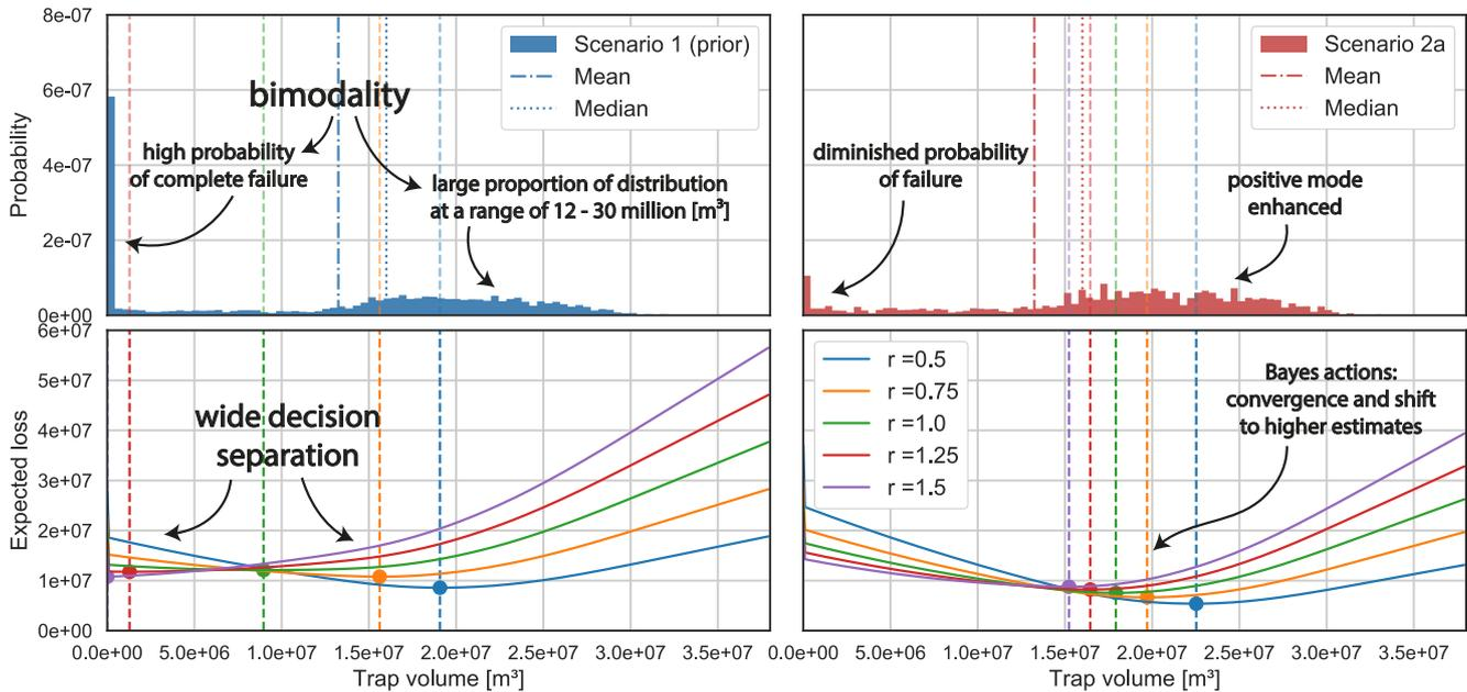
**Figure 5.** Trap volume distribution and resulting loss function realizations for Scenario 1 (prior) and Scenario 2a, where we introduced the likelihood of a thick seal. Comparing both, we can observe how the additional information reduced the bimodality in the posterior distribution (2a), particularly by reducing the probability of complete failure and enhancing positive probabilities. Consequently, Bayes actions converged and expected losses were reduced.
