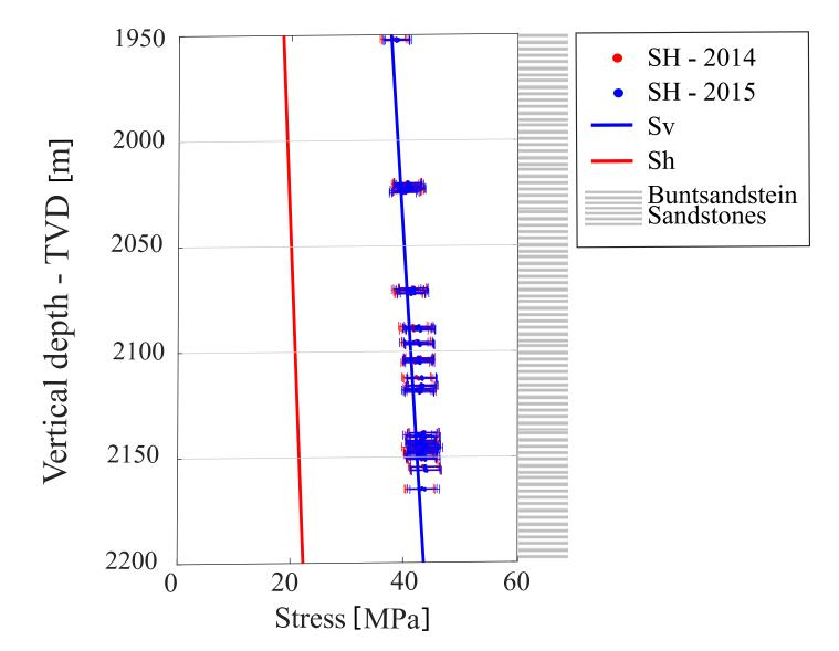
Figure 17: in-situ stress components Sh, SV and SH [MPa] in the deviated well GRT-2. SH stresses are inverted using a Mohr Coulomb failure criterion and represented as a function of the vertical depth (TVD) for the images acquired in 2014 and 2015. Error bars are calculated considering the errors on the measurements of the breakout widths, on the elastic parameters and on the Sh and Sv trends. The right column illustrates the lithological unit retained in the model.
