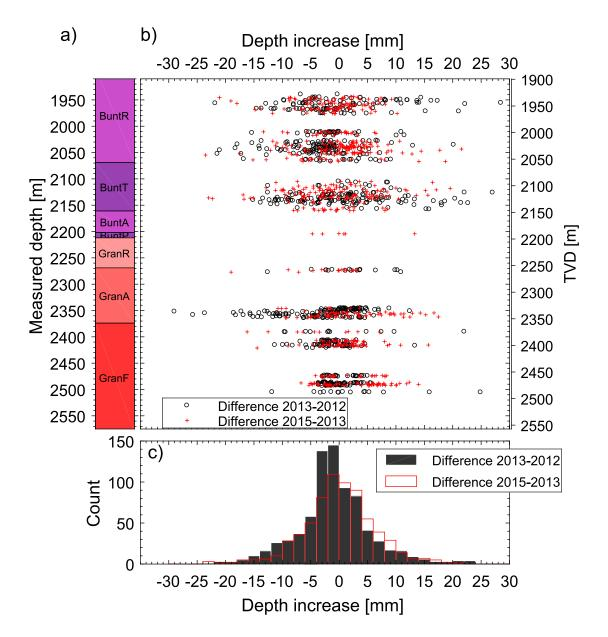
Figure 10: Evolution of the depth of the breakouts in the GRT-1 borehole in function of Measured Depth (MD) or Vertical Depth (TVD). a) Simplified lithologies along GRT-1 borehole (see Fig. 8 for the legend). b) Increase of the maximum radial extension between the 2012-13 time interval (black circles) and 2013-15 time interval (red crosses) presented in function of depth. c) histograms in 2 mm classes of breakout with changes for the 2012-13 interval (black) and 2013-15 interval (red).
