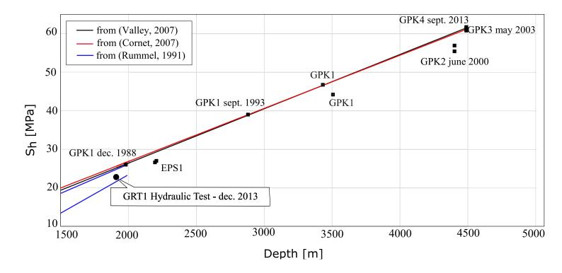
Figure 13: Minimal horizontal stress Sh [MPa] as a function of vertical depth (TVD) measured at the Soultz-sous-Forêts site from the analysis of high-volume injections in the GPK-1, GPK-2, GPK-3 and EPS-1 wells. The lower bound for the minimal horizontal stress Sh obtained from the analysis of the wellhead pressure measured during the stimulation of the well GRT-1 in Rittershoffen is represented for comparison as a black circle.
