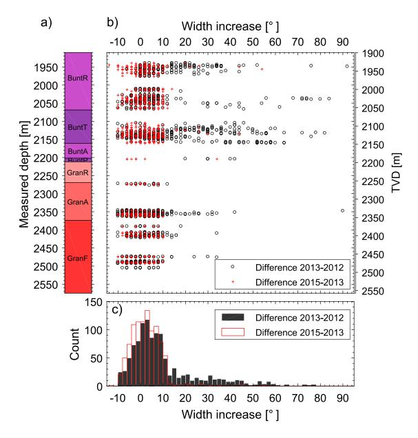
Figure 9: Evolution of breakout width in GRT-1 borehole in function of Measured Depth (MD) or Vertical Depth (TVD). a) Simplified lithologies along GRT-1 borehole (see Fig. 8 for the legend). b) Width increase between the 2012-13 time interval (black circles) and the 2013-15 time interval (red crosses) presented as a function of the vertical depth. c) histograms in  $2^{\circ}$  classes of breakout width changes for the 2012-13 interval (black) and the 2013-15 interval (red).
