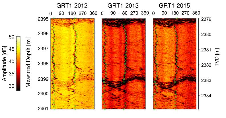
Figure 6: Examples of Drilling Induced Tension Fractures (DITFs), observed in the granitic section of GRT-1 in the amplitude images acquired in 2012, 2013 and 2015. The azimuth of the DITFs is measured every 20 cm (green crosses).
