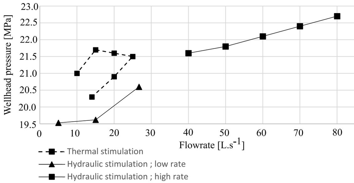
**Figure 12: Stabilized wellhead pressure [MPa] as a function of flow rate [ $\text{L}\cdot\text{s}^{-1}$ ], measured during the hydraulic stimulation of the GRT-1 well in 2013 (after Baujard et al., 2017).**
