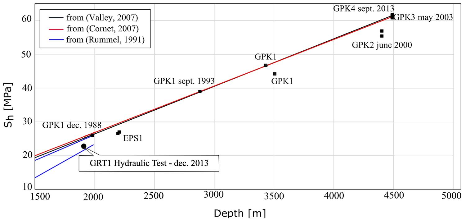
**Figure 13: Minimal horizontal stress  $S_h$  [MPa] as a function of vertical depth (TVD) measured at the Soultz-sous-Forêts site from the analysis of high-volume injections in the GPK-1, GPK-2, GPK-3 and EPS-1 wells. The lower bound for the minimal horizontal stress  $S_h$  obtained from the analysis of the wellhead pressure measured during the stimulation of the well GRT-1 in Rittershoffen is represented for comparison as a black circle.**
