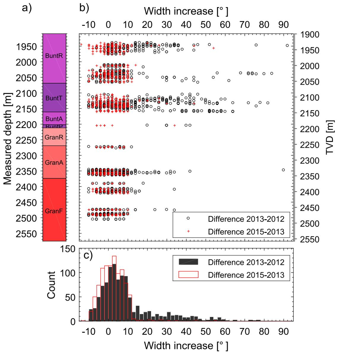
**Figure 9: Evolution of breakout width in GRT-1 borehole in function of Measured Depth (MD) or Vertical Depth (TVD). a) Simplified lithologies along GRT-1 borehole (see Fig. 8 for the legend). b) Width increase between the 2012-13 time interval (black circles) and the 2013-15 time interval (red crosses) presented as a function of the vertical depth. c) histograms in 2° classes of breakout width changes for the 2012-13 interval (black) and the 2013-15 interval (red).**
