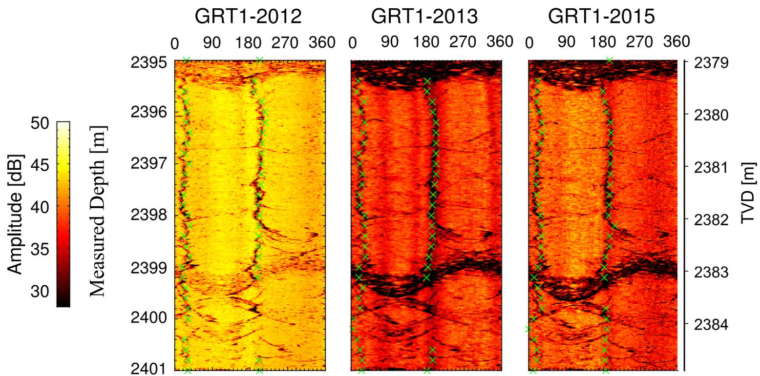
**Figure 6: Examples of Drilling Induced Tension Fractures (DITFs), observed in the granitic section of GRT-1 in the amplitude images acquired in 2012, 2013 and 2015. The azimuth of the DITFs is measured every 20 cm (green crosses).**
