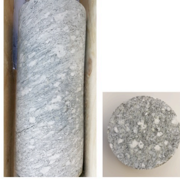
Figure 2: The Grimsel granite sample taken from the PRP1 borehole, with a diameter of 110 mm and a length of 240 mm. The nominal planes of stratification are inclined at about 50° to the axis of the sample.
