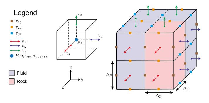
Figure 1. Staggered grid and location of variables.
