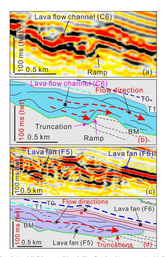
Figure 8: (a) and (b) Enlargement of the end of lava flow channel (ramp structure) and its line drawings; (c) and (d) Enlargement and its line drawings of the lava fans (F5 and F6). BM = base of volcano/lava flow. See locations in Figure 7.
