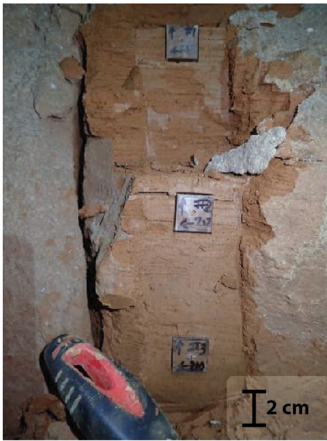
767 Figure 4: Example of clay sampling for the paleomagnetic study. Location at the entrance shaft (Highest 768 elevation of every samples (~580 m a.s.l.), Leicasse Cave system, Site 2, Fig. 1)
