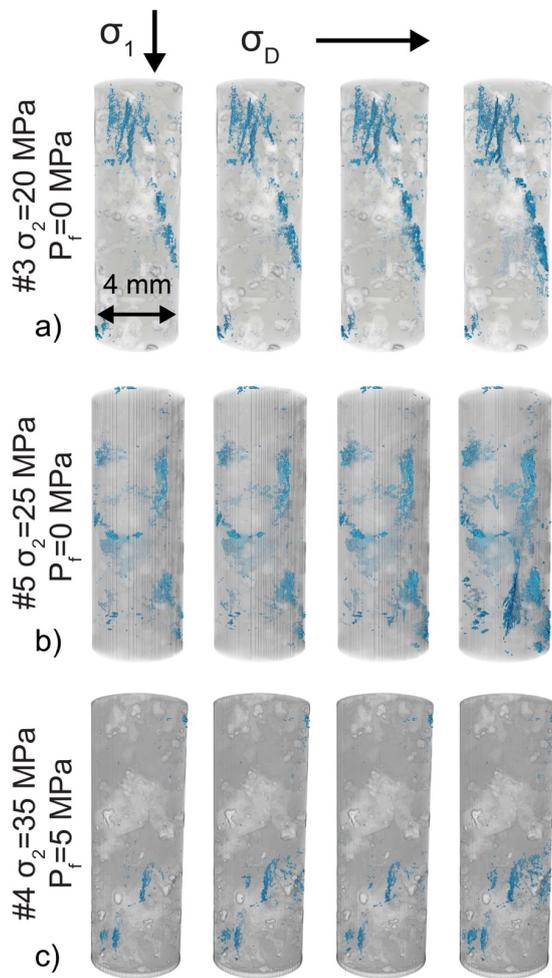
580 Figure 2: Evolving fracture networks in the final four loading steps of each experiment before system-size failure.
