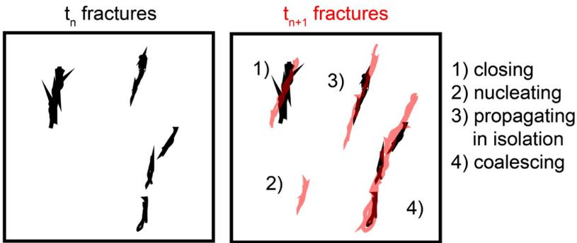
585 Figure 3: Modes of fracture network development captured by algorithm. By tracking individual fractures in sequential scans, we can identify fractures that 1) close, 2) nucleate, 3) propagate in isolation and 4) coalesce from one time to the next,  $t_n$  to  $t_{n+1}$ .
