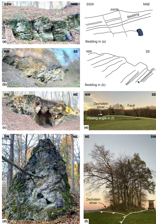
Figure 5. Photo panel of selected outcrops of Zechstein slivers along the Sontra Graben. The backpack is shown for scale. Approximate locations for each photo can be seen in Fig. 3.
