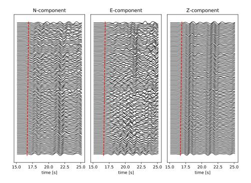
**Figure 3.** P-waveforms recorded by the nodal array, ordered by distance from the earthquake epicentre, band-pass filtered in the 0.5-1 Hz range, and scaled by the standard deviation of each trace. Time is relative to the start of the recordings, and is synchronised with the waveforms shown in Fig. 1. For reference, the move-out is indicated by the red dashed line.
