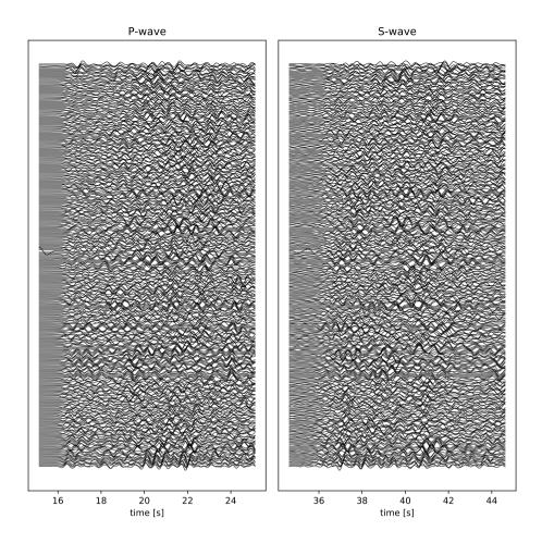
**Figure 6.** P- and S-waveforms recorded by the DAS array, ordered by distance from the earthquake epicentre, filtered in a 0.5-2 Hz pass band, and scaled by the standard deviation of each trace. Time is relative to the start of the recordings, and is synchronised with the waveforms shown in Fig. 1. For clarity, only every 20<sup>th</sup> channel waveform is plotted.
