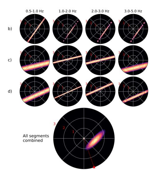
Figure 11. Beamforming results of the P-waveforms recorded on selected segments of the DAS array. In this figure, the panels show pseudopower  $\hat{P}$  normalised by the maximum power, such that  $0 \le \hat{P} \le 1$ , plotted as a function of the back-azimuth and apparent slowness of the candidate source. The slowness values (in s km<sup>-1</sup>) of the radial grid lines are as indicated by the red numbers. The letters indicated on the left of each row correspond to the panels in Fig. 10.
