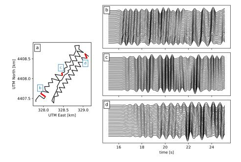
**Figure 10.** Location of the selected DAS cable segments, indicated in red in panel a. The corresponding P-waveforms that are shown in panels b, c, and d are filtered in a 0.5-2 Hz pass band and scaled by the standard deviation of each trace.
