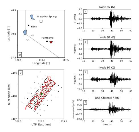
Figure 1. a) Location of the Brady Hot Springs natural laboratory and the March 2016  $M_L$  4.3 Hawthorne earthquake epicentre; b) Layout of the PoroTomo nodal seismometer array (black dots) and the fibre-optic cable (red line); c-e) Ground motions recorded on the N/E/Z-components of nodal seismometer #97, which is marked in panel b by a green dot; f) Strain rates recorded by a channel co-located with nodal seismometer #97. All waveforms are filtered in a 0.5-10 Hz pass band.
