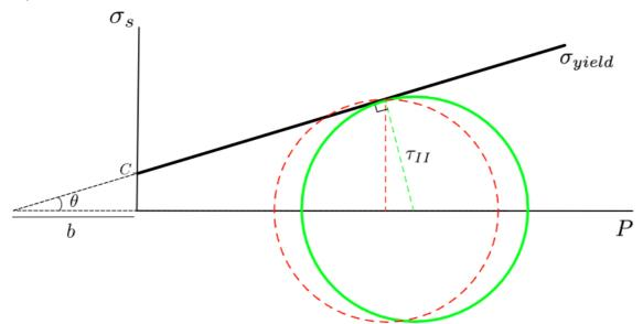
The plot shows the yield function (black) together with the Mohr-Circle (green circle, which has radius  $\tau_{II}$ ). At yielding (*F*=0), the Mohr-Circle exactly touches the yield stress function. This condition is *not*  $\tau_{II} = \sigma_{yield}$  (your eq. 4), as this gives the red circle (which predicts a stress that is somewhat larger than the yield stress). Instead, we can use trigonometry to compute the condition for *F*=0. If we define the effective angle of friction  $\theta$  as:
