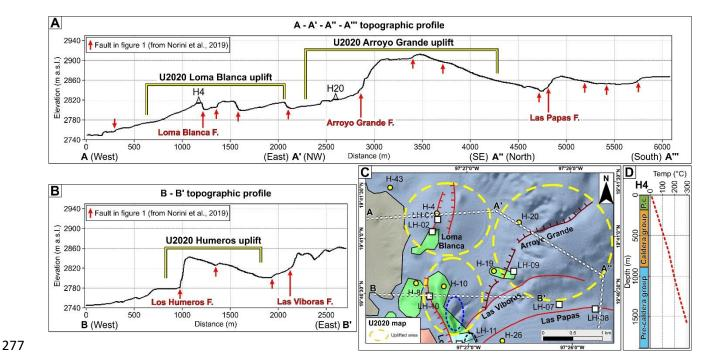
Figure 4: topographic profiles along the (A) A-A'-A''-A''' and (B) B-B' traces shown in Fig. 1, and (C) schematic geological map (modified from U2020) outlining the three uplifted areas discussed by U2020; the traces of the two topographic profiles and the locations of the H4 and H20 well are also shown. (D) H4 lithological and temperature log (well data from Arellano et al., 2003, and U2020). P.c.: Post-caldera group.
