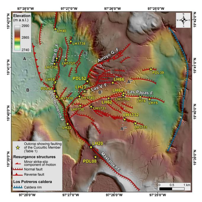
Figure 1: volcanotectonic map of the Los Potreros caldera area, on a DEM (illuminated from the E) (modified from GEMex, 2019 and Norini et al., 2019). Las V.F.: Las Viboras fault; Arroyo G.F.: Arroyo Grande fault; Loma B.F.: Loma Blanca fault. Location of outcrops in Fig. 2 and Tab. 1 is shown. Traces of A–A'–A''–A'' and B–B' topographic profiles of Fig. 4 are also shown.
