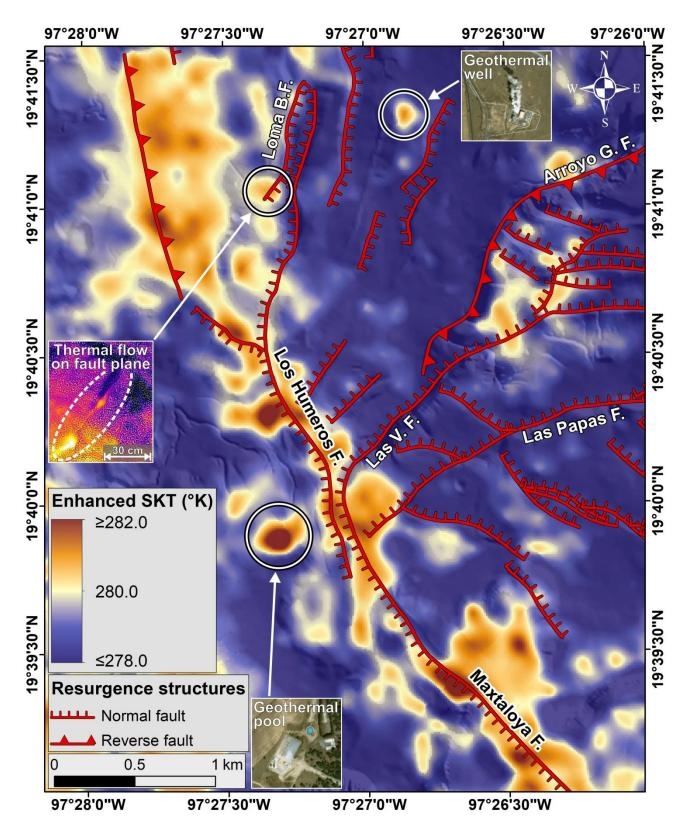
Figure 3: enhanced surface kinetic temperature (SKT) of the Los Potreros caldera obtained from ASTER AST08 night-time thermal remote sensing data (see Norini et al., 2015, for details on methods and results). Examples of field-validated sources of thermal anomaly are shown in the insets (Norini et al., 2015, 2019). Thermal satellite data: credits LP-DAAC, USGS EROS data center at the NASA. Satellite images in the insets: credits Esri, DigitalGlobe, GeoEye.
