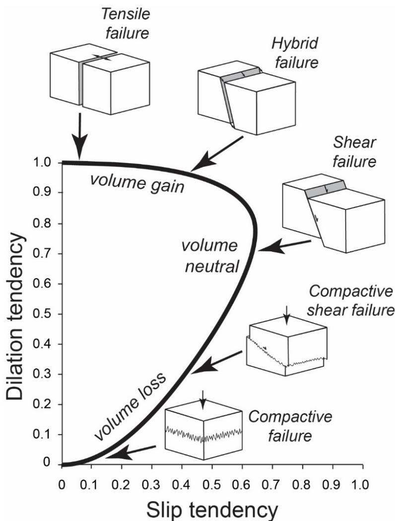
**Figure 1.** General graphical relationship between maximum slip tendency and dilation tendency, and associated rock failure
