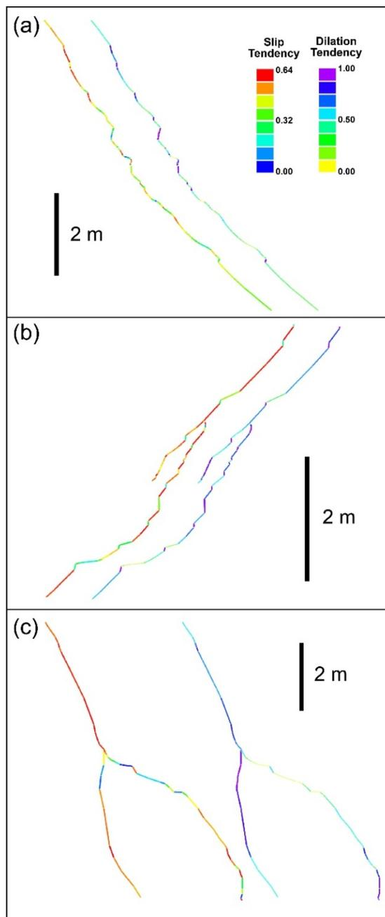
175 **Figure 4.** Slip tendency (left profile of each pair) and dilation tendency (right profile of each pair) profiles of the (a) Textbook, (b) Spanish Goat, and (c) Big Indigo faults at Sycamore Bluffs using the inverted stress tensor described in the text and illustrated in terms of slip tendency and dilation tendency in **Fig. 3**. Although these plots are similar to those presented in Ferrill et al. (2017a), they have been updated to reflect the inverted stress state shown in **Fig. 3**.
