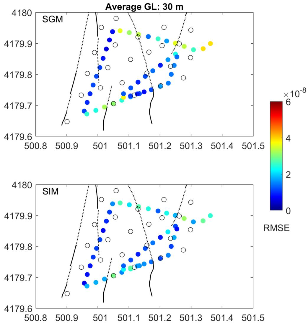
**Figure S4:** Misfits between the array derived strain and the DAS strain data (volcanic explosion on 6 July 2019) after increasing the gauge length to 30 m using a simple average.
