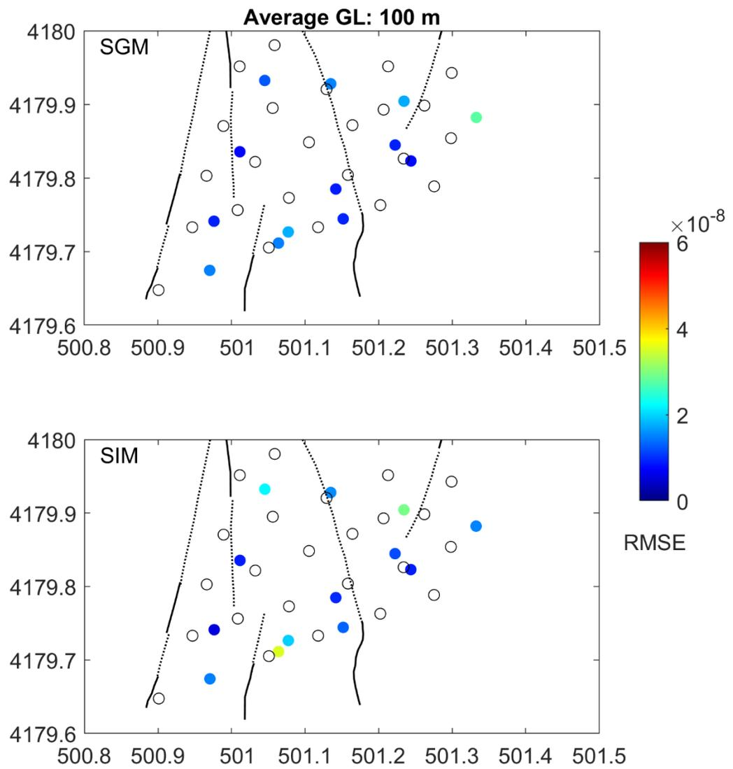
**Figure S7:** Misfits between the array derived strain and the DAS strain data (volcanic explosion on 6 July 2019) after increasing the gauge length to 100 m using a simple average.
