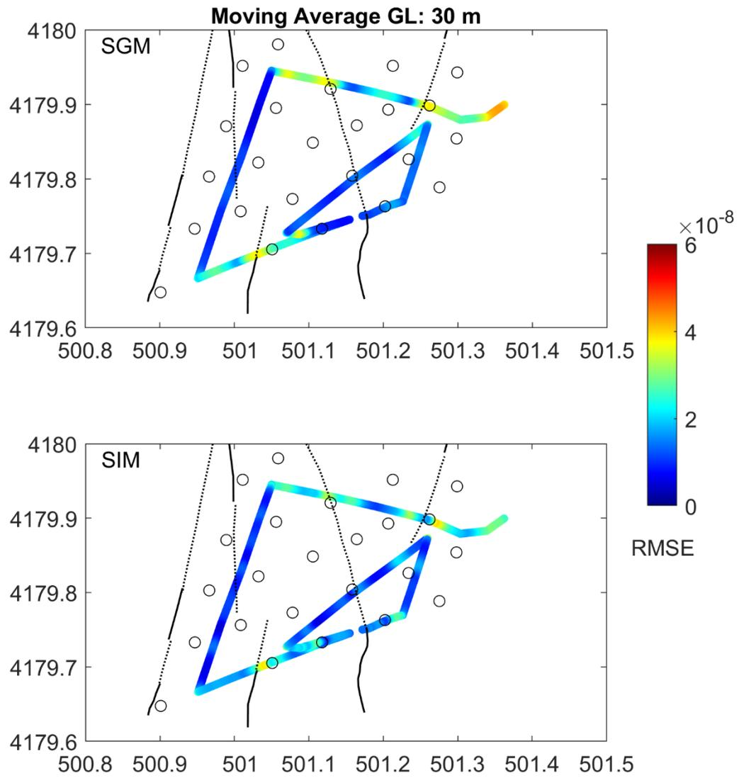
**Figure S5:** Misfits between the array derived strain and the DAS strain data (volcanic explosion on 6 July 2019) after increasing the gauge length to 30 m using a moving average.
