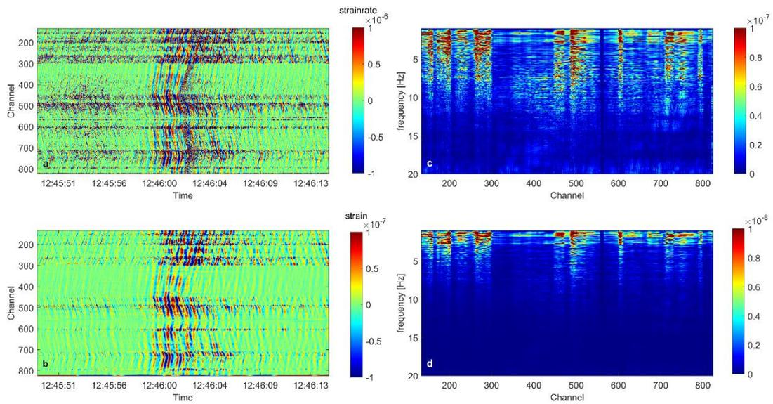
**Figure S1:** Time series (a, b) and spectra (c, d) during a small volcanic explosion (VE) at Etna on 6 July 2019. (a) Raw DAS strainrate; (b) strain computed by integrating over time the raw strainrate data; (c) spectra of the raw strainrate DAS records overall the channel; (d) spectra of strain records.
