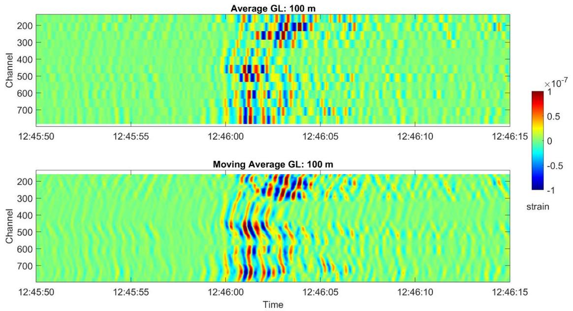
**Figure S6:** Strain data (volcanic explosion on 6 July 2019) after increasing the gauge length to 100 m. Two methods were used: (top) averaging the data every 50 channels (100 m); (bottom) averaging with a mobile mean over 50 channels with a shift of 1 channel.
