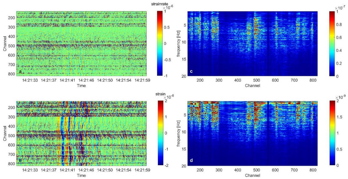
**Figure S2:** Time series (a, b) and spectra (c, d) during an LP event (LP) at Etna on 27 August 2019. (a) Raw DAS strainrate; (b) strain computed by integrating over time the raw strainrate data; (c) spectra of the raw strainrate DAS records overall the channel; (d) spectra of strain records.
