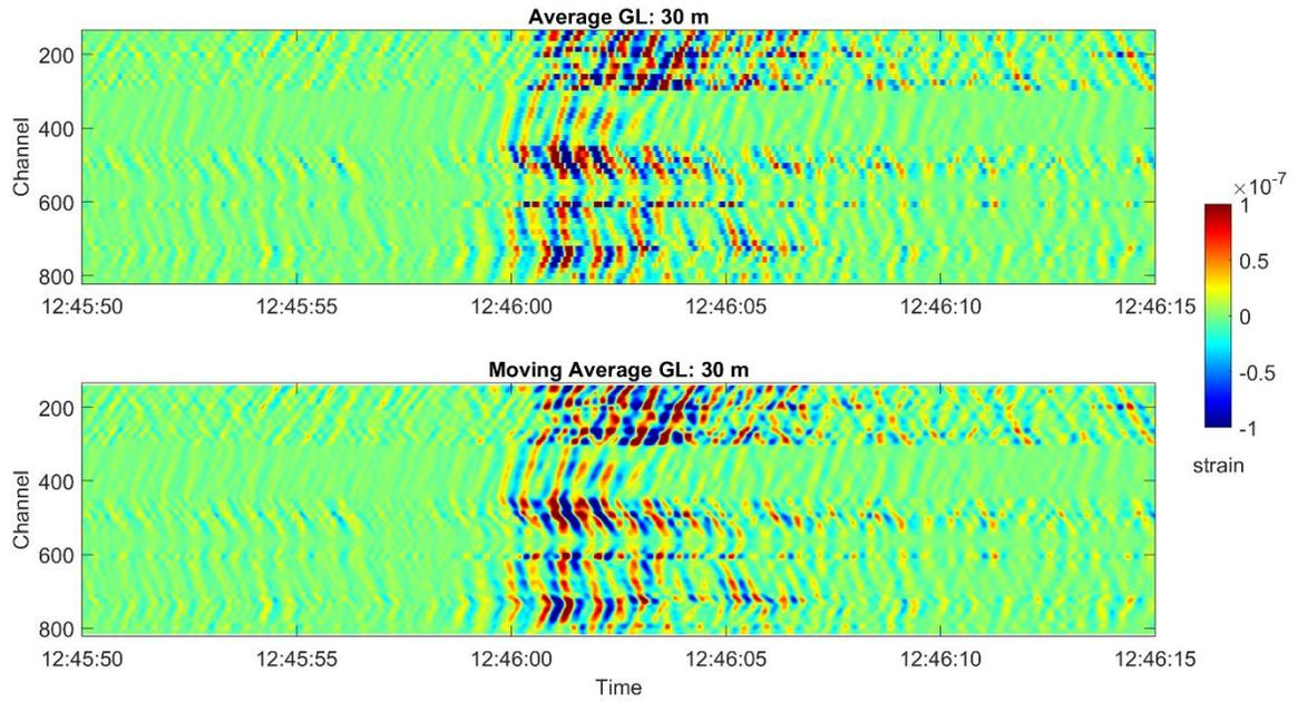
**Figure S3:** Strain data (volcanic explosion on 6 July 2019) after increasing the gauge length to 30 m. Two methods were used: (top) averaging the data every 15 channels (30 m); (bottom) averaging the data with a mobile mean over 15 channels with a shift of 1 channel.
