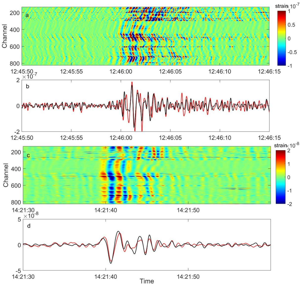
350 **Figure 2:** Time series of DAS strain during a small volcanic explosion (VE) at Etna on 6 July 2019 (a, b) and during a long-period (LP)
