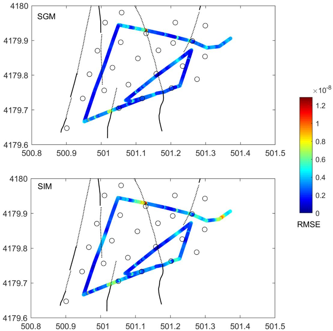
**Figure 4:** RMSE residuals between DAS strain measurements (Fig. 2c) and the strain derived from the seismic array along the fibre for the LP event.
