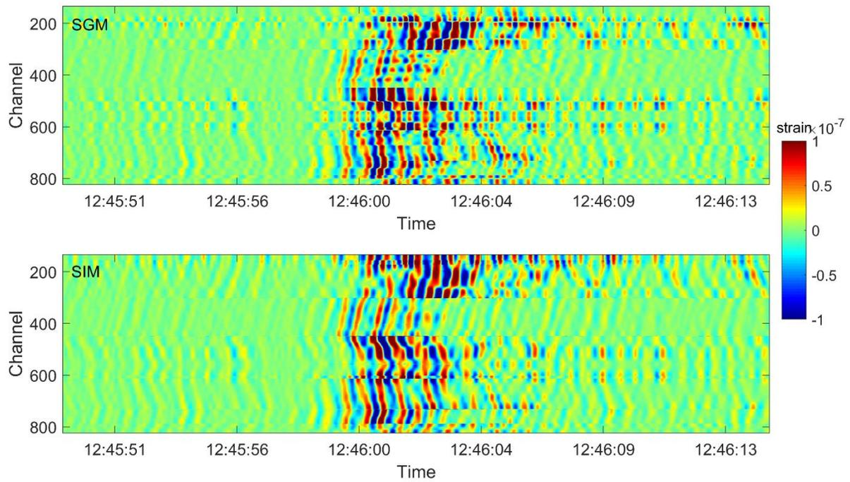
380 **Figure 7:** – Strain estimates over all fibre channels using SGM (top) and SIM (bottom) for the VE event. The solutions with the minimum
