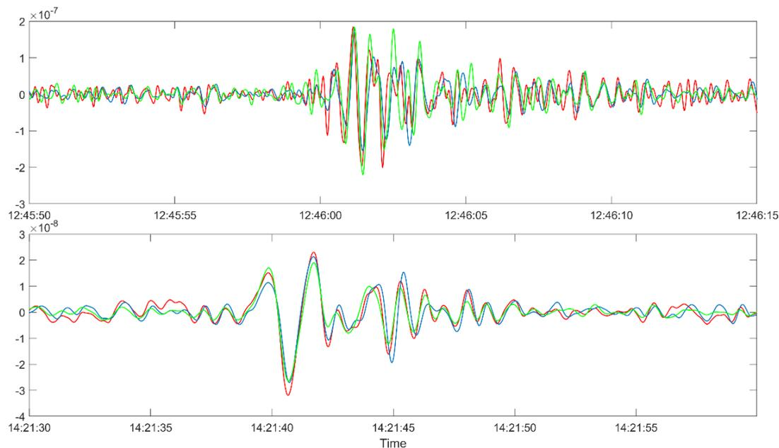
**Figure 6:** Array-derived strain estimates at station Bb04 (Fig. 1) using the SIM (green line) and the SGM (blue line) in comparison with DAS strain data (red line). Computations are performed for the VE (top) and LP (bottom) events.
