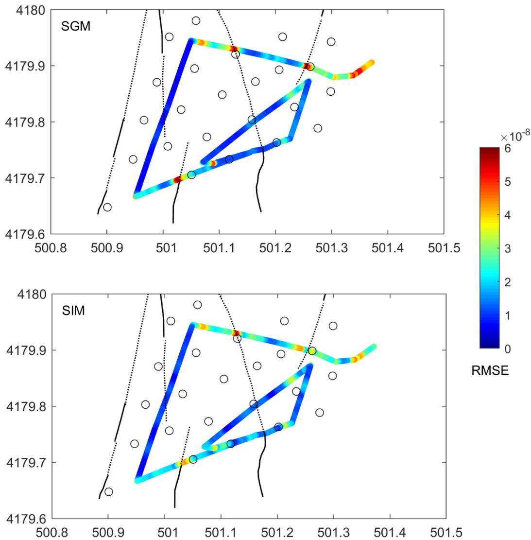
**Figure 3:** RMSE residuals between DAS strain measurements (Fig. 2a) and the strain derived from the seismic array along the fiber for the VE event. (Top) DAS vs. the seismo-geodetic method (SGM). (Bottom) DAS vs. the spatial interpolation method (SIM). Black lines and open circles indicate faults and seismometers shown in Fig.1, respectively. For more details see text.
