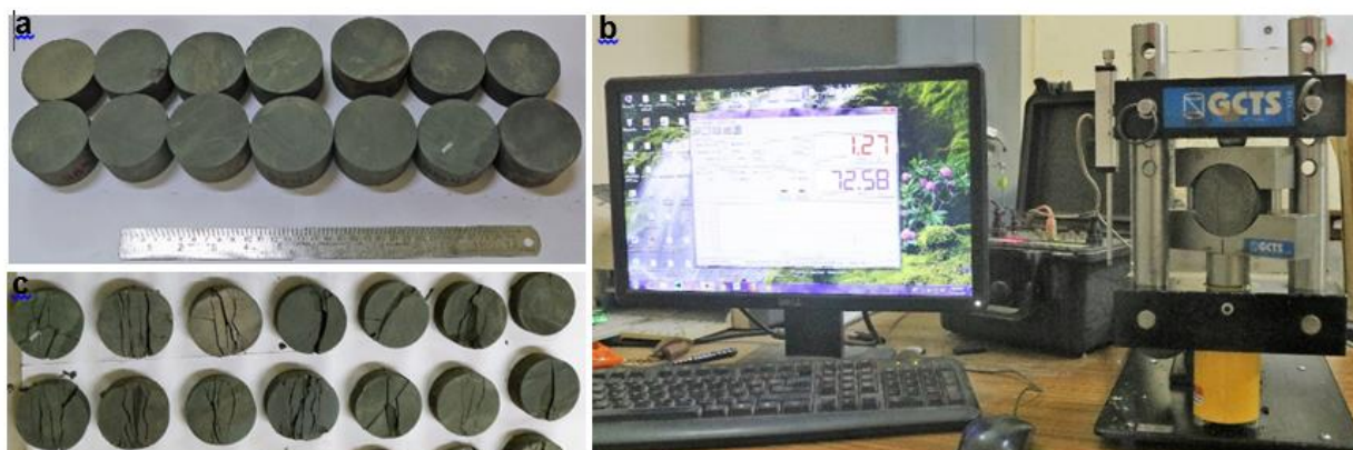
Figure 06. Tensile strength determination of metabasalt samples. (a) Sample cores for Brazillian tensile strength (BTS) determination. Diameter: length=2:1. (b) Instruments used for measuring BTS. (c) Sample cores obtained after failure.
