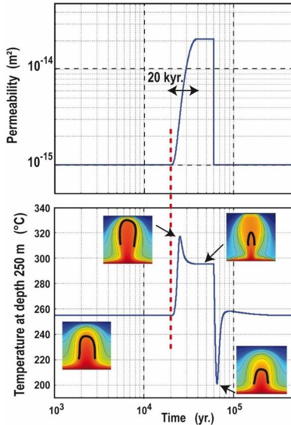
260 **Figure 4.** Effect of a time-dependent permeability, increasing by a factor of 20 in 20 kyr. The finger-like geometry (lower left pattern) evolves towards a bulb-like geometry (upper right pattern). Temperature profile (bottom plot) shows short-duration heating and cooling events. The thick black contour on convective patterns corresponds to the 300°C isotherm. . Color-bar (not shown) is the same as in previous figures.
