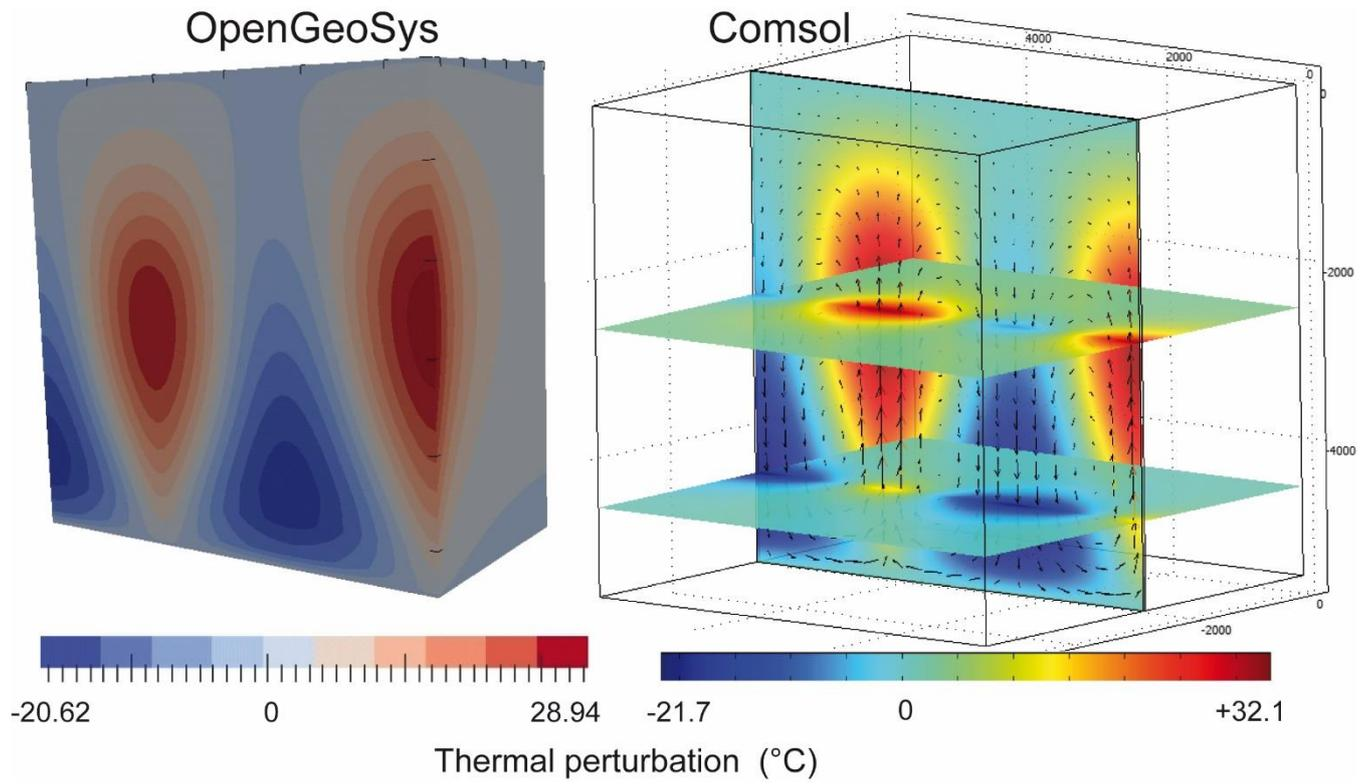
**Figure B1.** Benchmark experiment for a 40 m wide fault zone embedded in impervious host rock (cube of 5.5 km), as in the Magri et al. (2017) study (left). Our result (right) indicates slight differences in temperature perturbation (see text) but convective pattern is identical.
