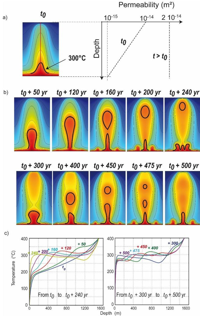
**Figure 7. Instantaneous increase of the medium permeability (from  $10^{-14} \exp(-z/650)$  at  $t = t_0$ , to  $2 \cdot 10^{-14} \text{ m}^2$ , at  $t > t_0$ ) resulting in a high velocity upwelling, where the central blob does not lose much energy during ascent. a) Steady-state triangular-like upwelling**
