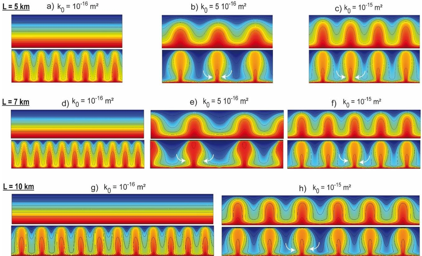
305 Figure 6. Additional experiments illustrating thermal inheritance for 3 distinct box lengths  $L$ . Initial ( $t = t_0$ ) thermal regimes
