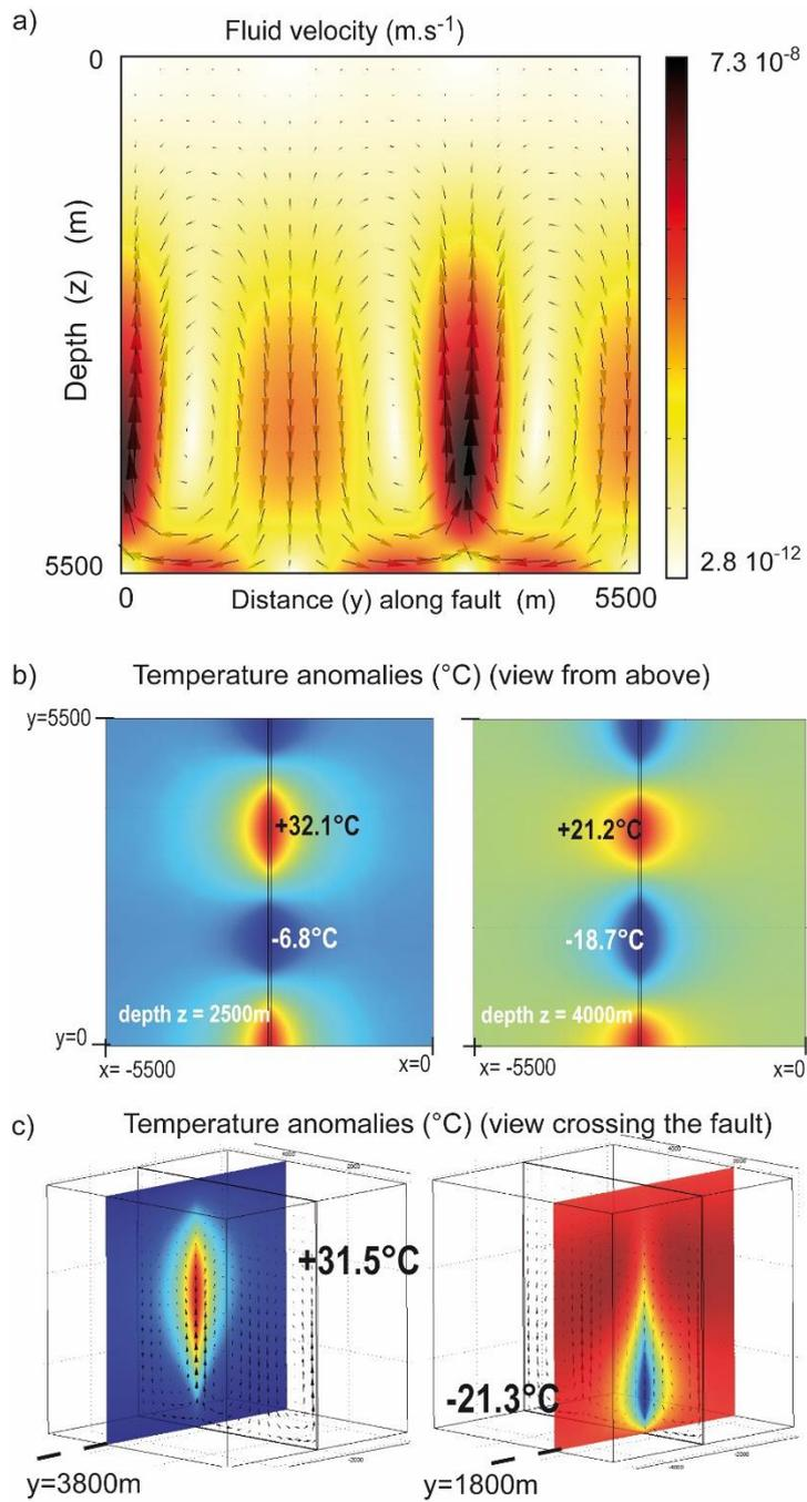
765 **Figure B2.** Details on the 3D benchmark experiment of Figure B1. a) Field velocity and values within the fault ; b) lateral diffusion of temperature anomalies at depths 2500 and 4000 m ; c) lateral diffusion of hot and cold anomalies, perpendicularly to the fault.
