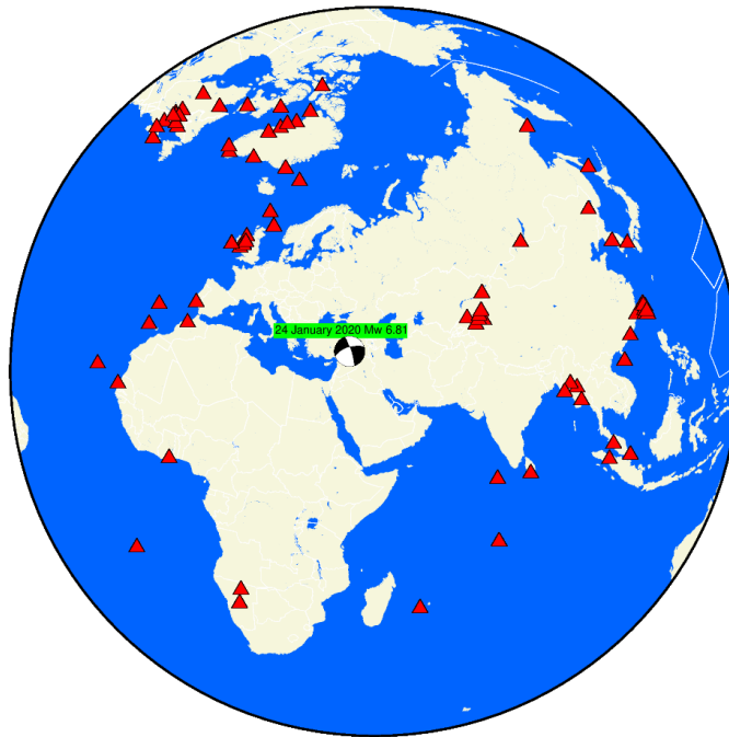
Figure S2. Distribution of 76 teleseismic broadband stations at distances of 30-80 degrees (red triangles). Focal mechanism of the 24 January 2020 Mw 6.8 Elazığ-Sivrice earthquake. The mechanism coordinate denotes the epicenter.
