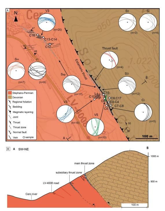
Figure 2: (A) Geological map and (B) cross-section of the Estamariu thrust, which juxtaposes a Devonian unit against a Stephano-Permian sequence (H=V, no vertical exaggeration). Lower-hemisphere equal-area stereoplots of the Devonian bedding (S<sub>0</sub>), regional foliation (Sr), thrust zone foliation affecting the hanging wall (SD) and footwall (SSP), magmatic layering (Sm) and the different faults and veins observed in the study area are also included. Location in Fig. 1B.
