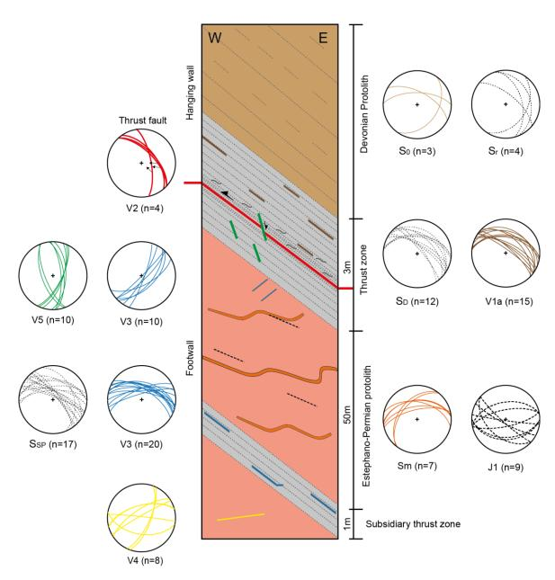
815 Figure 3: Sketch showing the spatial distribution of mesoscale structures within the main outcrop and lower-hemisphere equalarea stereoplots of the different mesostructures.
