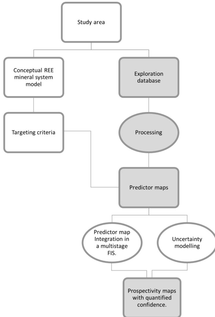
**Figure 2: Flow chart depicting the methodology. Rectangular boxes contain generated objects, and oval boxes contain processes used for creating the objects. Shaded boxes indicate the objects and processes created and implemented in a GIS, respectively.**
