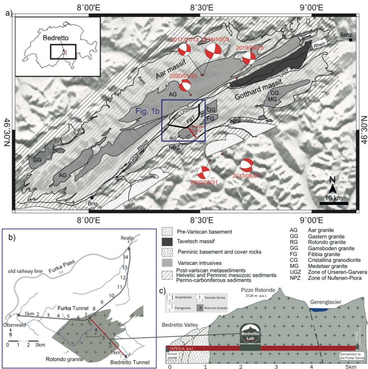
**Figure 1:** a) Integrated geological, topographical and seismological information near the Aar and Gotthard massif surrounding the Bedretto Lab (Keller and Schneider, 1982; adapted from Lützenkirchen and Loew, 2011, and Gischig et al., 2020). b) Map view of the Bedretto Tunnel and the hosting Rotondo granite. c) Cross-sectional view of the Bedretto Lab with respect to the tunnel.
