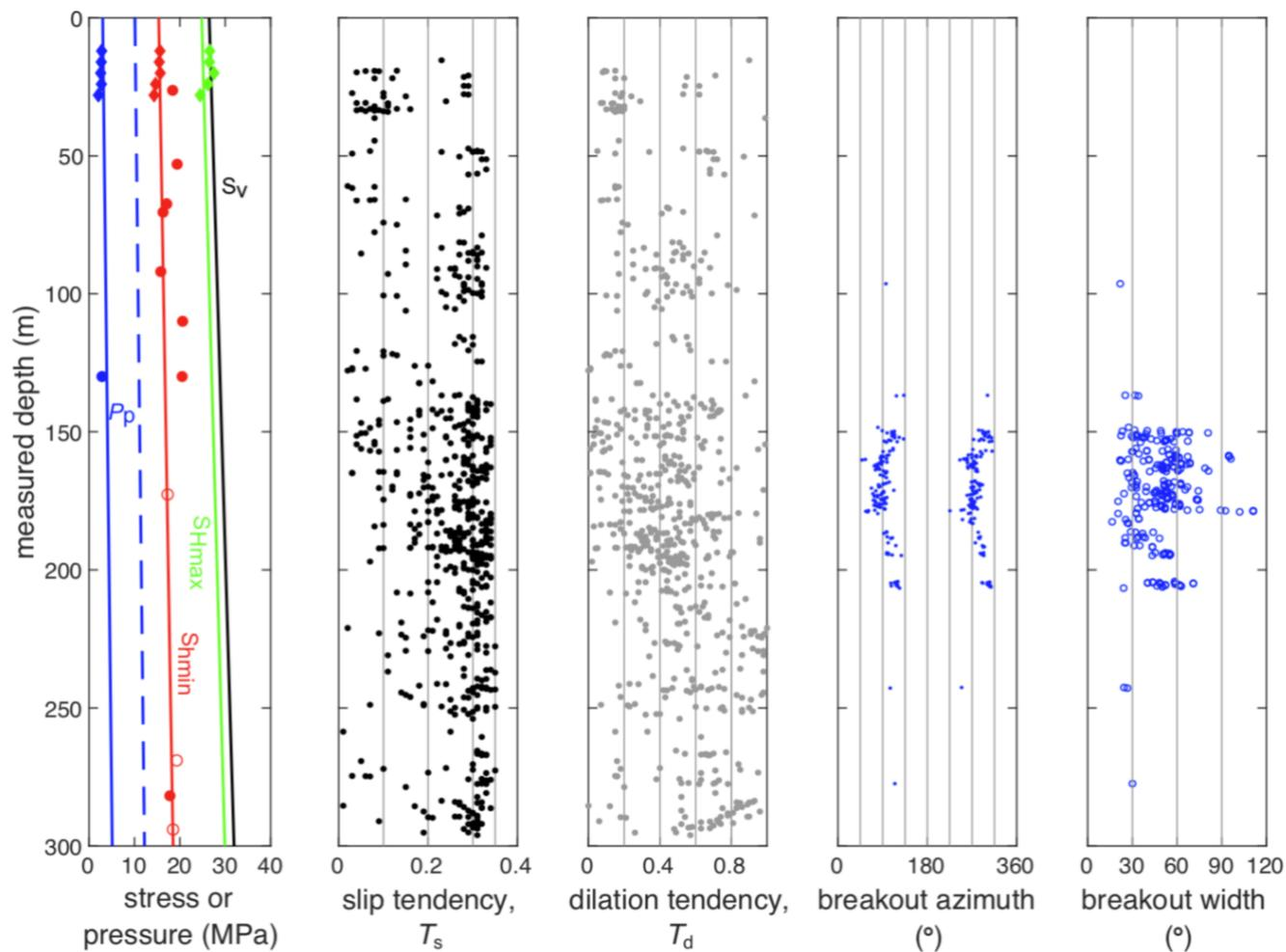
835 **Figure 8: Integrated geomechanical information of borehole CB1: stress and pore pressure profiles (Diamonds are from SB borehole data; circles are from CB1, while open circles are of uncertainty; dashed blue gradient represents hydrostatic pore pressure.); slip tendency ( $T_s$ ) and dilation tendency ( $T_d$ ) of all mapped structures (shown in Figure 5); breakout azimuths and widths ( $0^\circ$  refers to the high-side of the borehole).**
