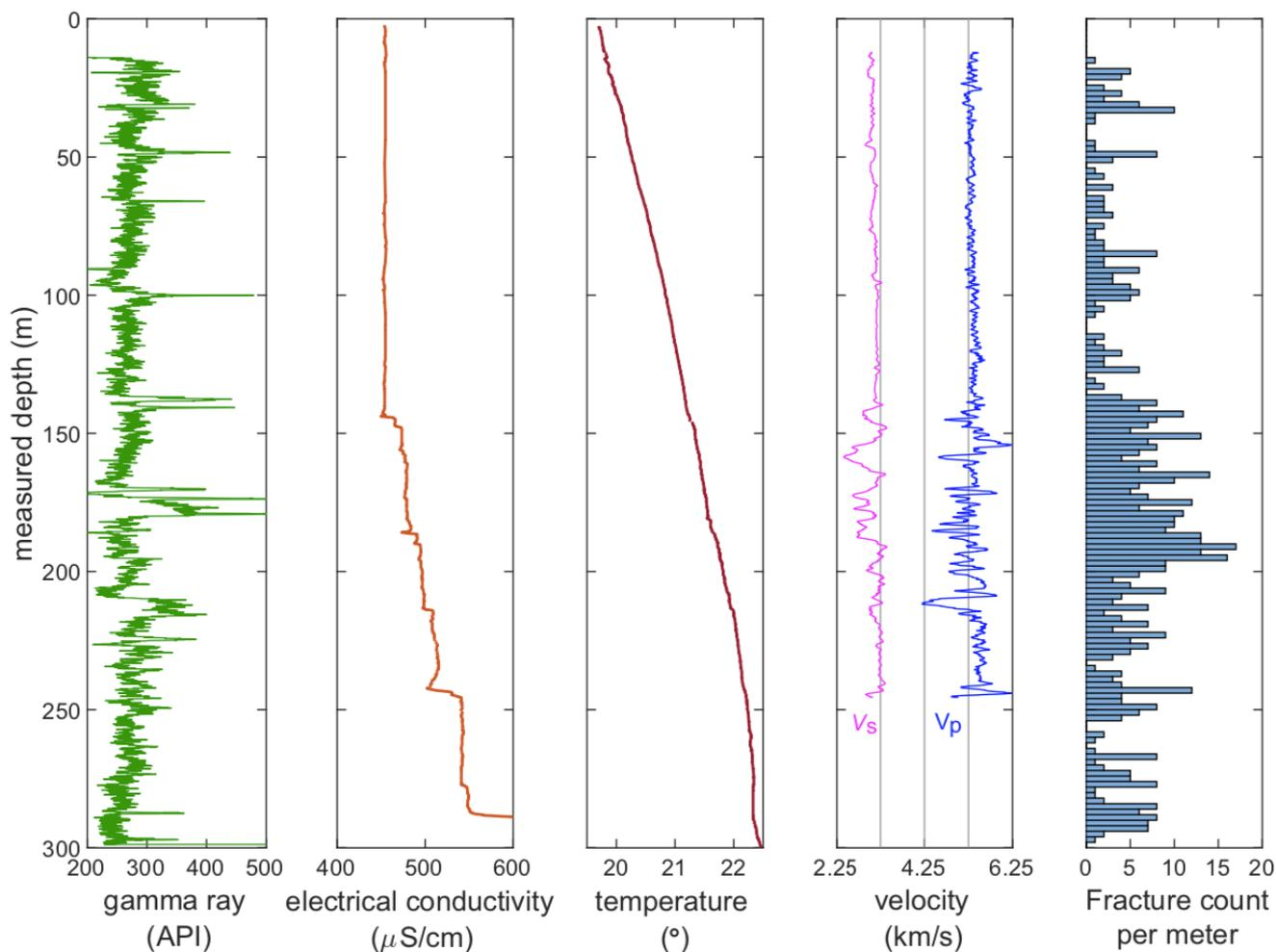
**Figure 4:** Integrated geophysical logs of borehole CB1: gamma ray; electrical conductivity; temperature; sonic compressional and shear wave velocities ( $V_p$  and  $V_s$ ); density of mapped fractures from televiewer logs.
