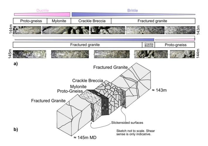
Figure 6: a) Core images, compositions and the structure of the major fault zone encountered in borehole CB1 (between 143-145 m measured depth). Ductile and brittle structures can be seen in close proximity to each other. Brittle structures are located at the boundaries of ductile features; b) Schematics of the fault zone structure.
