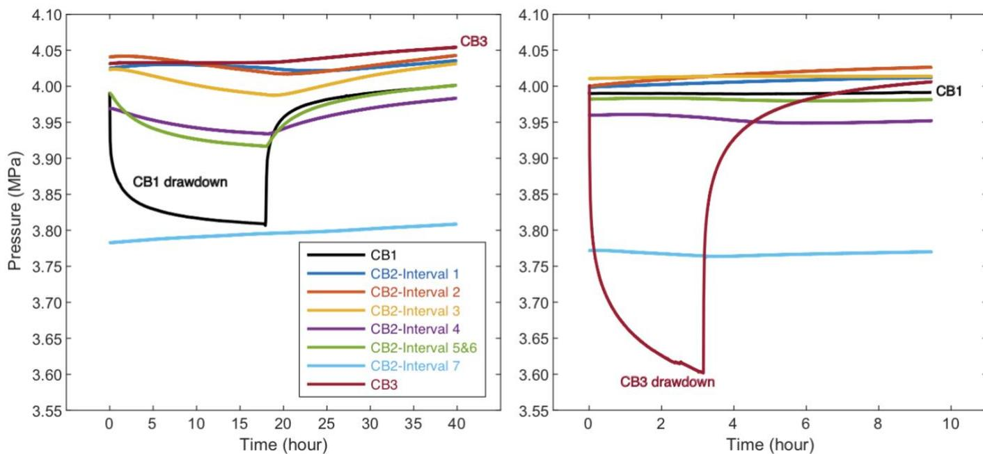
Figure 10: The pressure response of boreholes/intervals to the drawdown in CB1 (left) and CB3 (right).
