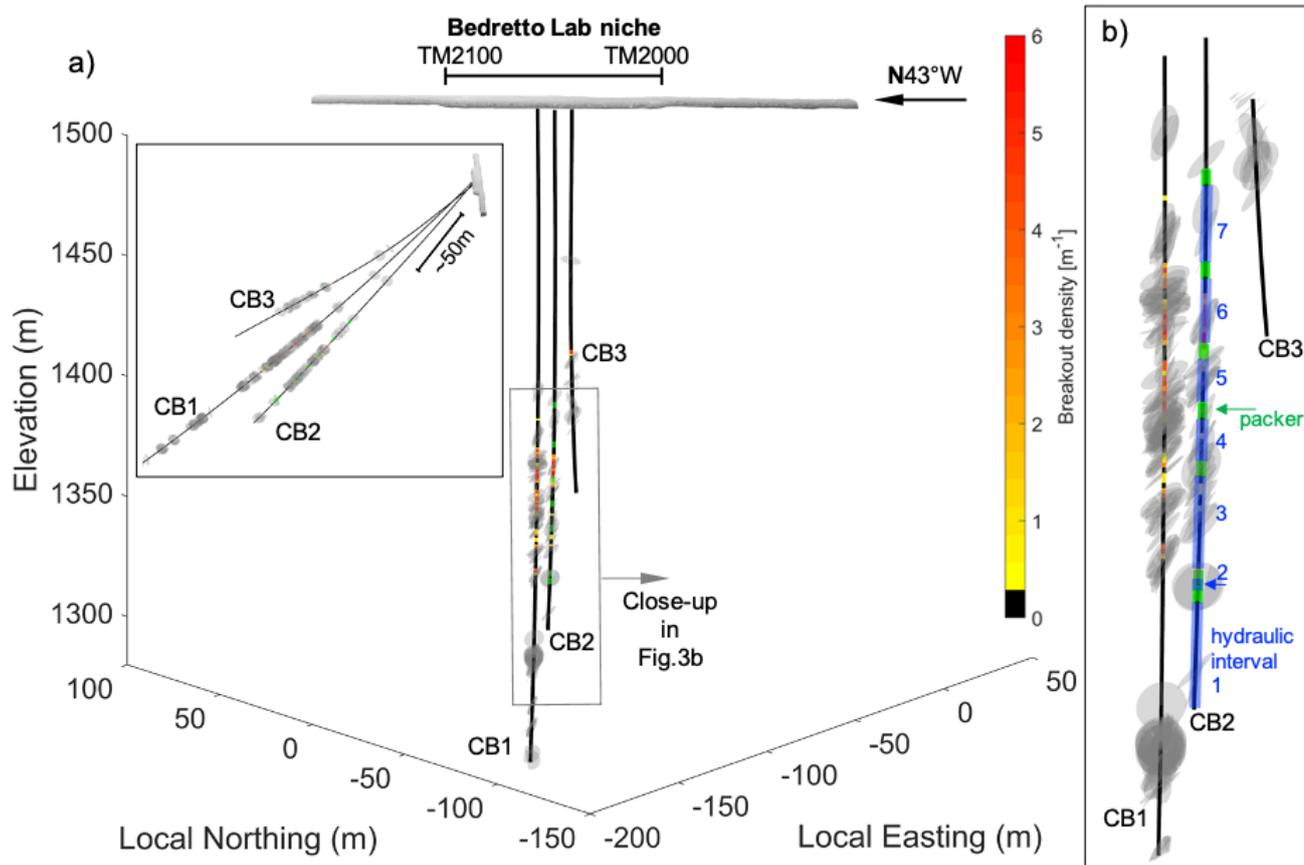
805 **Figure 3: Configuration of boreholes CB1,2,3 and the mapped major fractures/fault zones therein. a) Looking down approximately normal to the three boreholes. Inset shows the side view of the boreholes. b) Close-up of the major fault zone interval. Note the breakout density along the CB borehole major fault zone and the multi-packer system (and the divided hydraulic intervals) installed in CB2 (see Table 2 for details).**
