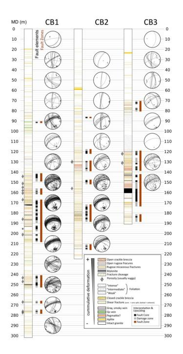
Figure 5: Core description showing the geological designations and structural orientations (measured by the acoustic and optical televiewers, i.e., ATV/OTV).
