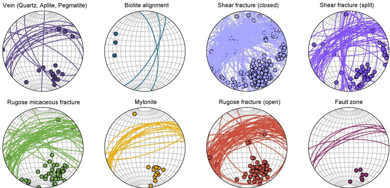
830 **Figure 7: Mapped geological structures by type. The upper row shows the orientation of structures that are mainly ‘closed’ (based on visual examination of the cores). The lower row shows the orientations of structures with higher shear strain and can be perceived as ‘open’. Note the structures shown in the lower row are almost exclusively oriented NE-SW.**
