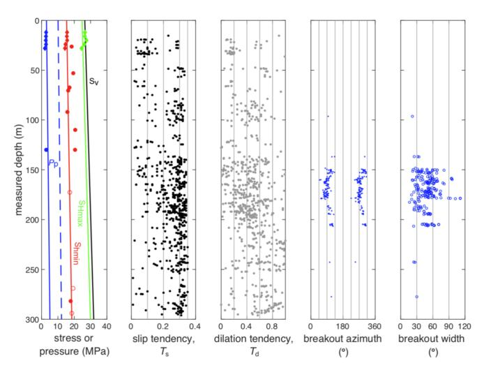
835 Figure 8: Integrated geomechanical information of borehole CB1: stress and pore pressure profiles (Diamonds are from SB borehole data; circles are from CB1, while open circles are of uncertainty; dashed blue gradient represents hydrostatic pore pressure.); slip tendency ( $T_s$ ) and dilation tendency ( $T_d$ ) of all mapped structures (shown in Figure 5); breakout azimuths and widths ( $0^\circ$  refers to the high-side of the borehole).
