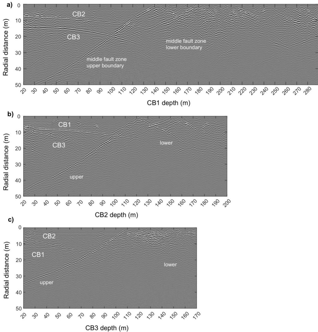
**Figure 9: Single-hole GPR reflection profiles (100 MHz) along: a) CB1, b) CB2, and c) CB3. From each borehole, the nearby boreholes are identified (and labelled) as prominent reflectors. The middle unit of major fault zones are clearly visible.**
