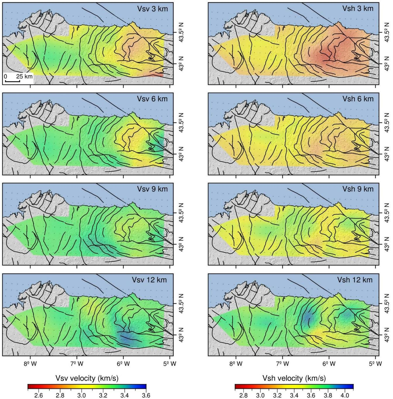
920 **Figure 6:** Inverted  $V_{sv}$  (left panels) and  $V_{sh}$  (right panels) velocity tomographic maps for depths of 3, 6, 9 and 12 km. Black lines represent the main Alpine and Variscan faults. The point grid marks the position of each inverted  $V_s$  depth model.
