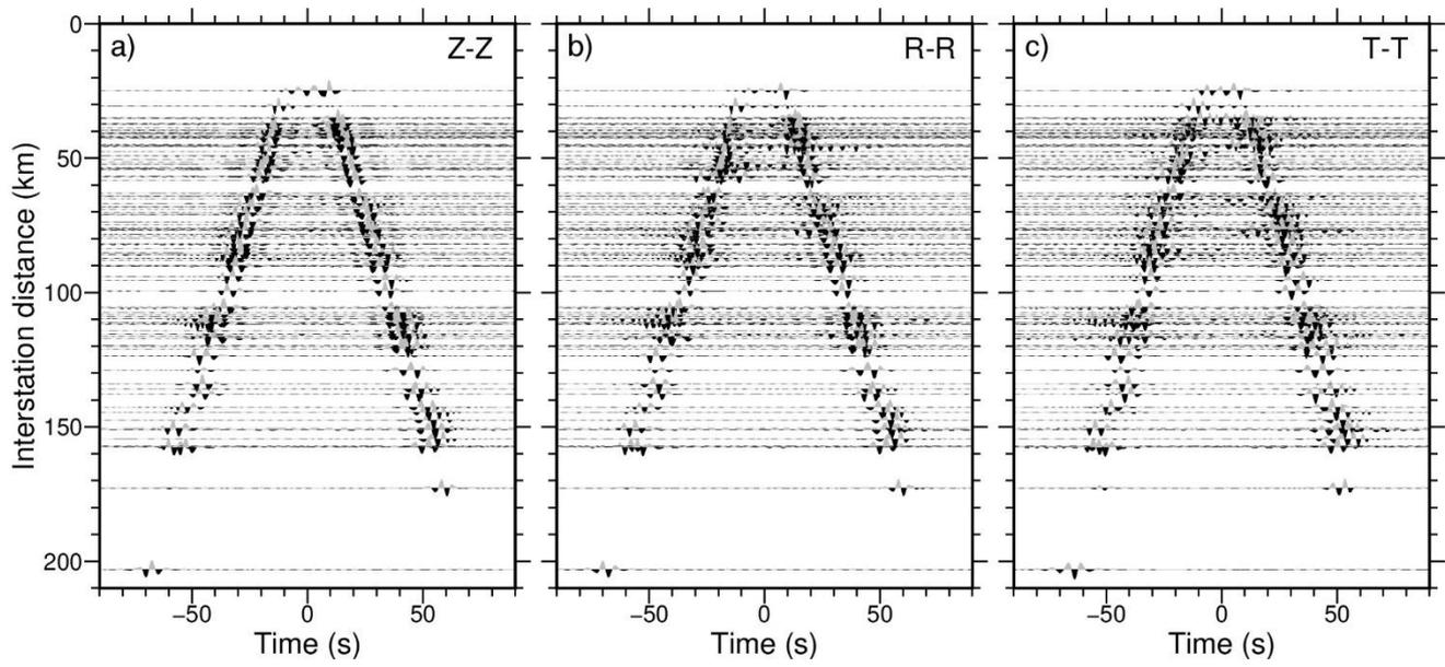
905 **Figure 3: Record sections showing the EGFs of all the available station pairs obtained from the cross-correlation of the a) vertical (Z-Z), b) radial (R-R) and c) transverse (T-T) components.**
