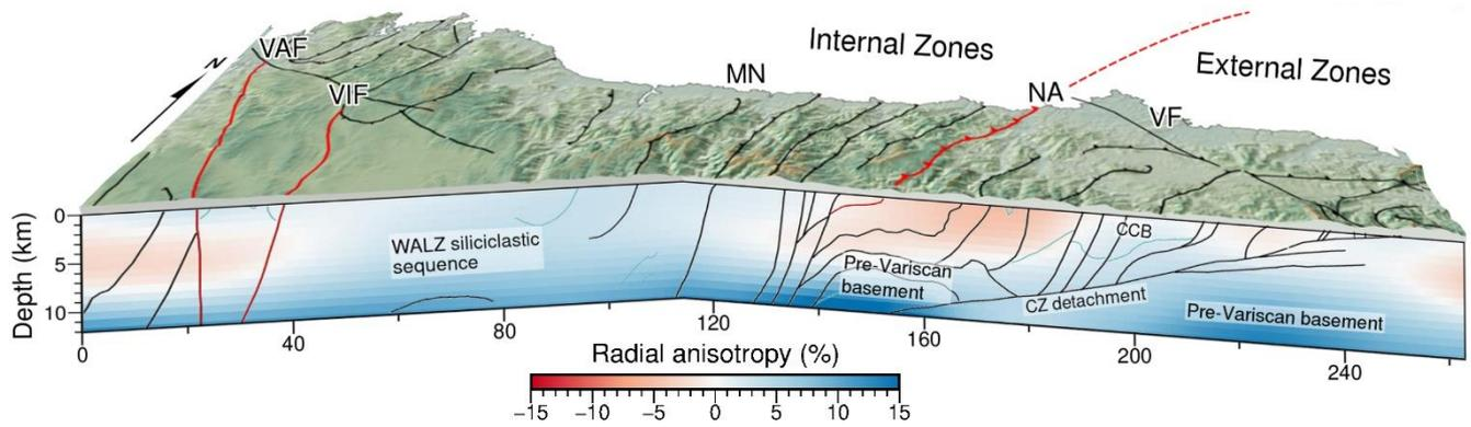
945 | **Figure 109:** Schematic 3D block showing the upper-crustal radial anisotropy variation across an E-W transect of the upper crust in NW Iberia. The main structural features are superimposed, based on Pérez-Estaún et al. (1991). Red lines indicate the structures that bound the main Variscan domains displayed in Fig. 1. The location of the cross-section is highlighted in Fig. 1a. CCB: Central Coal basin, VF: Ventaniella fault, MN: Mondoñedo nappe, VIF: Vivero fault, VAF: Valdoviño fault.
