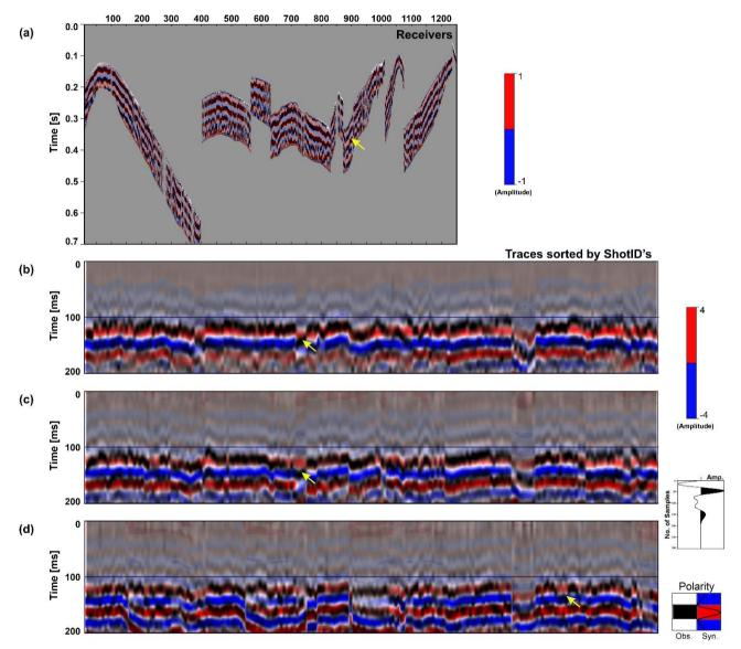
Figure 7: (a) Data fitting comparison between observed data (black and white) and synthetic data (red and blue) produced from FWI velocity model (Fig. 5b) for a common-shot gather. (b), (c) and (d) shows common-offset (CO) sections for bin-centered at 500 m, 1000 m and 1500 m. Source wavelet used during FWI is shown on the bottom right. The overall fitness of the data is acceptable,
