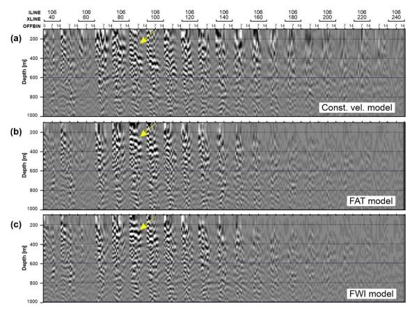
Figure 12: Surface offset gathers for (a) constant velocity model, (b) FAT model, and (c) FWI model for a selected inline (106, the same as in Fig. 10) shown for every 20<sup>th</sup> crossline. Offset varies between 0-1400 m. Improvement in focusing and flatness of the reflector is marked by the yellow arrow.
