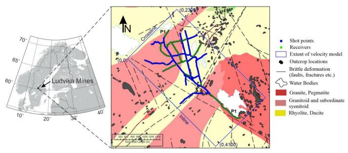
Figure 1: 3D data acquisition geometry at Blötberget and bedrock geology (modified after Geological Survey of Sweden). Receivers and shots of the sparse 3D survey are shown by green and blue dots. The rectangular blue box shows the extent of velocity model space used for FWI and subsequent depth imaging using RTM in local coordinates.
