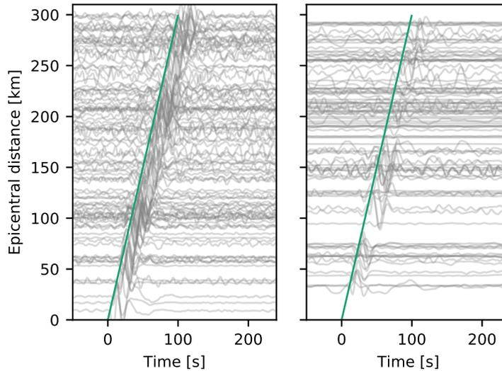
**Figure 3.** Vertical component seismograms of permanent AASN stations, sorted by distance. (left) 2017-03-06, Mw 4.1, Switzerland, (right) 2017-10-27, Mw 3.6, France. Time in seconds after origin time. Waveforms bandpass filtered between 0.02 and 0.07 Hz. Rayleigh waves dominate the seismograms in this frequency range with an average phase velocity of 3 km/s (green line).
