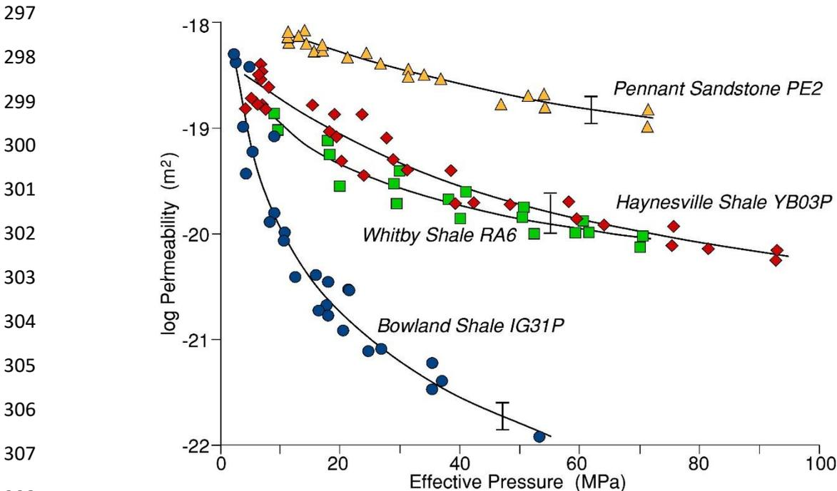
309 **Figure 3: Matrix permeability of Pennant sandstone for flow normal to bedding, and for Bowland and Haynesville**
