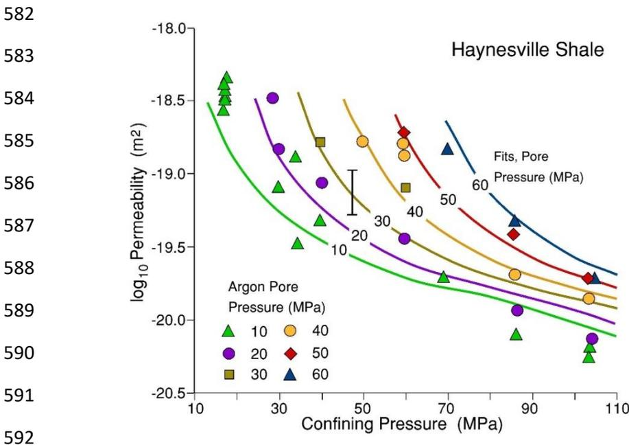
593 **Figure 11: Permeability of Haynesville Shale versus total confining pressure for various values of constant gas pore**
