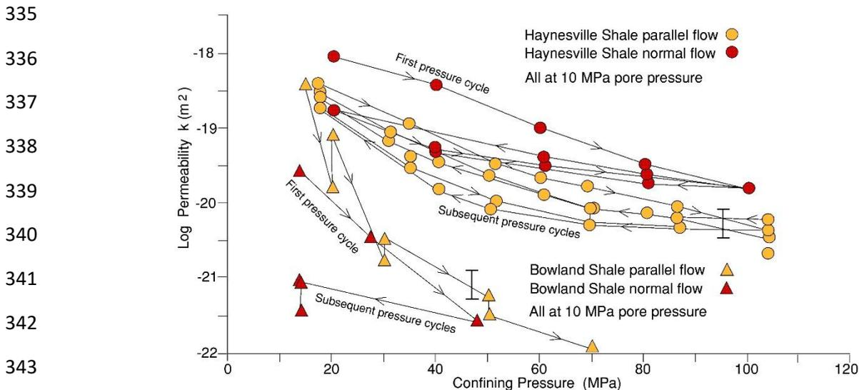
344 **Figure 4: Comparison of data at 10 MPa pore pressure for flow parallel and normal to layering in the two shales.**
