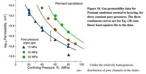
down to the micron scale, in the Pennant sandstone the greater part of the rock volume is not porous, as it
