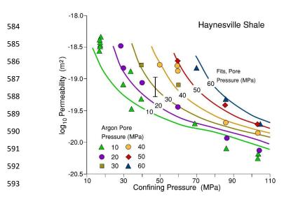
Figure 11. Permeability of Haynesville Shale versus total confining pressure for various values of constant
