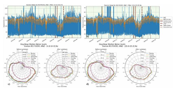
**Figure 11:** Temporal changes in seismic noise observed at the station located on the 8th floor of the Unirea Hotel in Focsani in the frequency bands 4-14 Hz (a) and 15-25 Hz (b). Lockdown effects are shown on 24-hour clock plots in the frequency bands 4-14 Hz (c) and 15-25 Hz (d, see Figure 1 for the station location).
