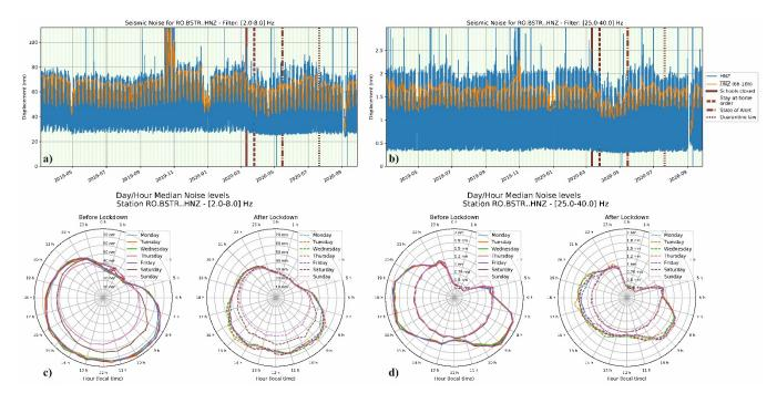
**Figure 4:** Lockdown effects on seismic noise in downtown Bucharest (BSTR): top - Evolution of DRMS for the March 2019 - September 2020 period based on displacement data in the bands 2-8 Hz (a) and 25-40 Hz (b); bottom - 24-hour clock plots showing average displacement variation for each day of the week and for the period before lockdown and during lockdown for the bands 2-8 Hz (c) and 25-40 Hz (d). The location of the station is displayed in Figure 1.
