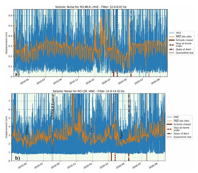
**Figure 12:** Long-term changes of seismic noise at MLR (a) and CJR (b) stations located in remote places less populated. Note the comparable minimum noise level during the UNTOLD Festival and Orthodox Easter or Christmas holidays at CJR station. The locations of the stations are displayed in Figure 1.
