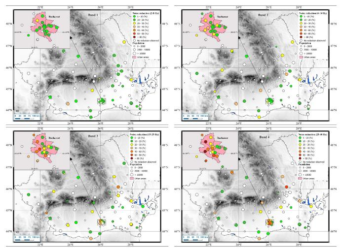
**Figure 2:** Percent change in DRMS during the period March 25-April 23, 2020 (right after the stay-at-home order entered into force) with respect to the interval February 10 - March 10, 2020 in the frequency bands a) 2-8 Hz (Band 1); b) 4-14 Hz (Band 2); c) 15-25 Hz (Band 3) and d) 25-40 Hz (Band 4).
