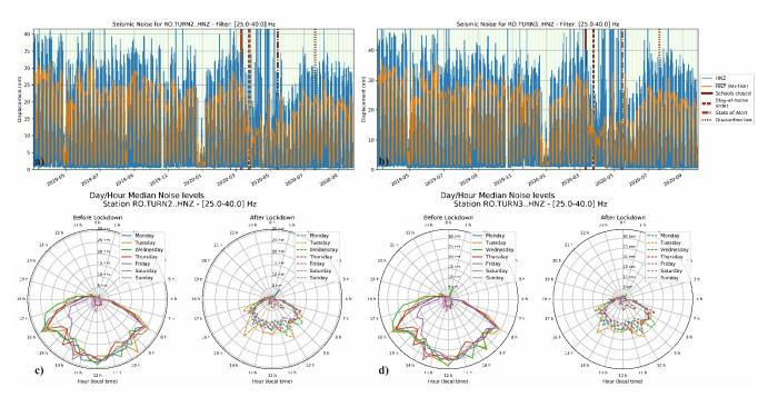
**Figure 10:** Temporal changes in seismic noise observed at the station located on the 6th (a) and 10th (b) floors of the IAP building. Lockdown effects are shown on 24-hour clock plots for both stations in (c) and (d, see Figure 1 for the station location).
