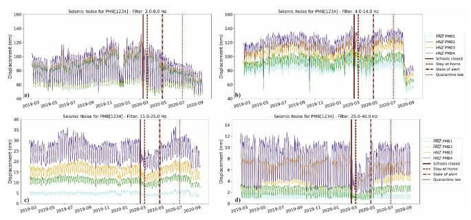
**Figure 8:** Long-term DRMS variations at the stations located in the Bucharest City Hall building observed in the frequency bands 2-8 Hz (a), 4-14 Hz (b), 15-25 Hz (c) and 25-40 Hz (d). Note the higher noise levels in the lower frequency bands as well as the significant increase of the noise levels at the stations deployed from the ground floor to the top of the building (see Figure 1 for the station location).
