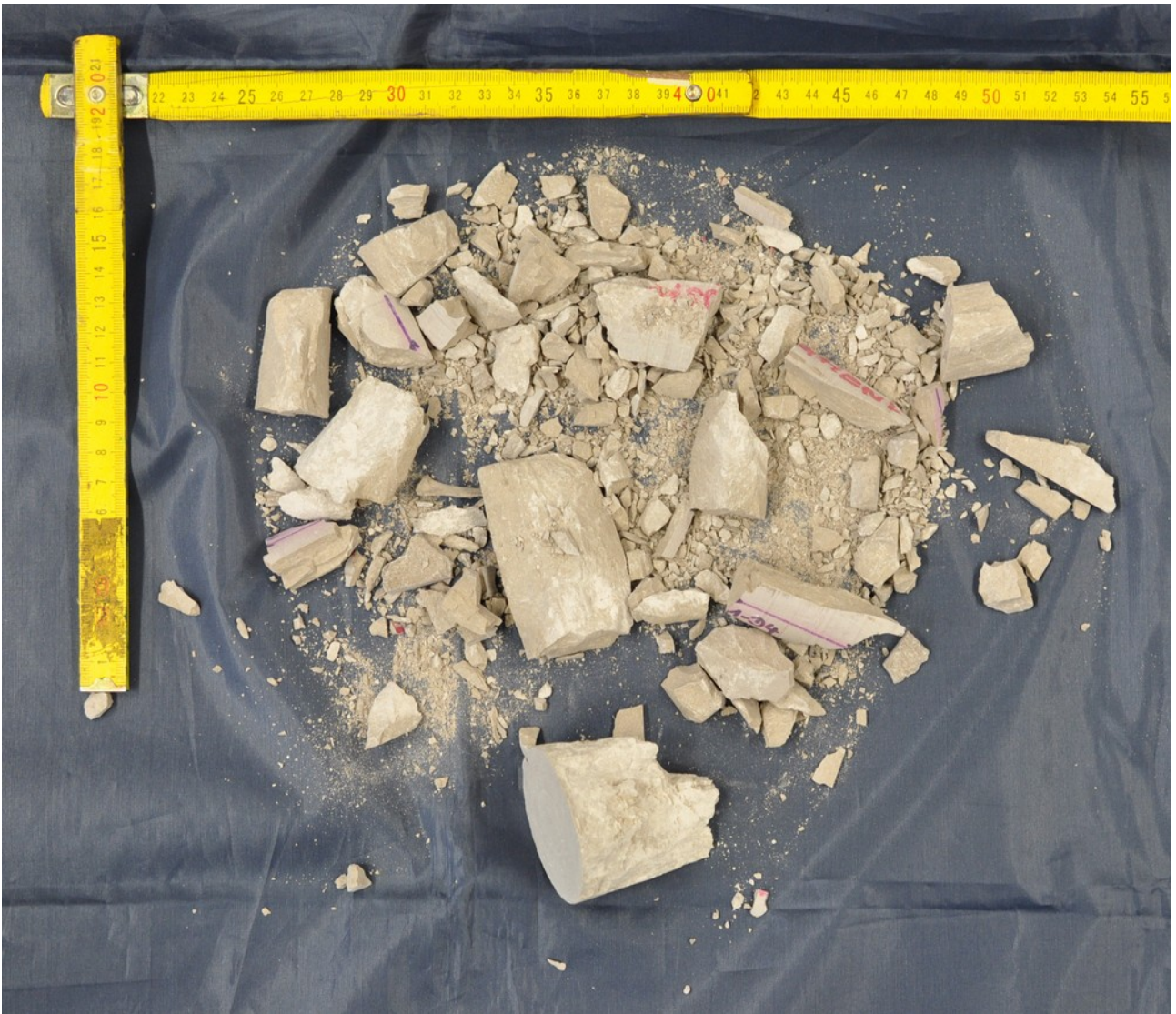
Figure 3: Fragments of a limestone sample after a triaxial deformation experiment.
