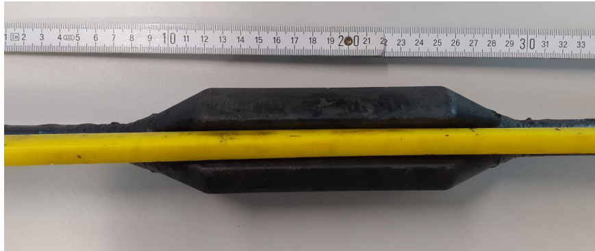
158 159 Figure 1: Down-hole cable configuration of the sucker rod with a centralizer (black) and the fiber-optic cable 160 (yellow)
