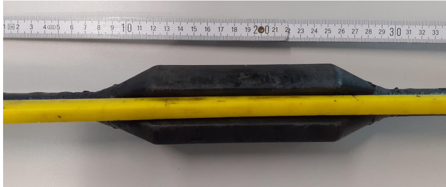
157 158 Figure 1: Down-hole cable configuration of the sucker rod with a centralizer (black) and the fiber-optic cable 159 (yellow)
