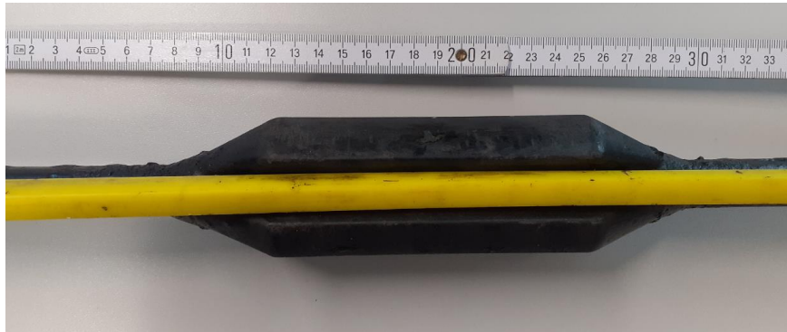
159 160 Figure 1: Down-hole cable configuration of the sucker rod with a centralizer (black) and the fiber-optic cable 161 (yellow)
