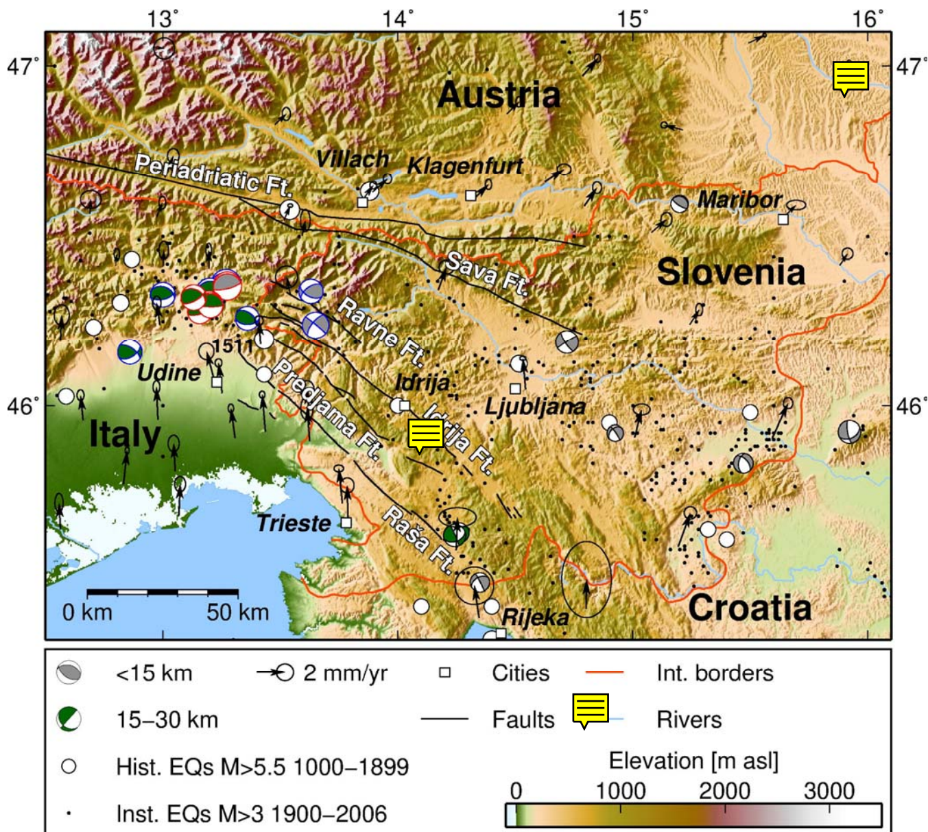
95 Figure 1: The study area in the Alps-Dinarides transition zone. Main faults of interest (black lines) are from Moulin et al. (2016) and own mapping. Historical and instrumental seismicity are from the SHEEC database (Stucchi et al., 2013; Grünthal et al., 2013); the 1511 Idrija EQ is marked (note that the location is uncertain, the earthquake probably occurred either on the Idrija Fault or on the SW side of the mountain front in Italy). Beachballs with black outlines are derived from p-wave arrivals (Herak et al., 1995); those with blue outlines are from quakes M>5 determined from first arrivals used in the Italian RCMT catalogue 1997-2017 (Pondrelli et al., 2002 and updates thereof); red outlines mark data from teleseismic body waveform inversion 1953-1984 (Anderson and Jackson, 1987). GPS data are from Metois et al. (2015) in a Eurasia-fixed reference frame. Topography is from SRTM1 data.
