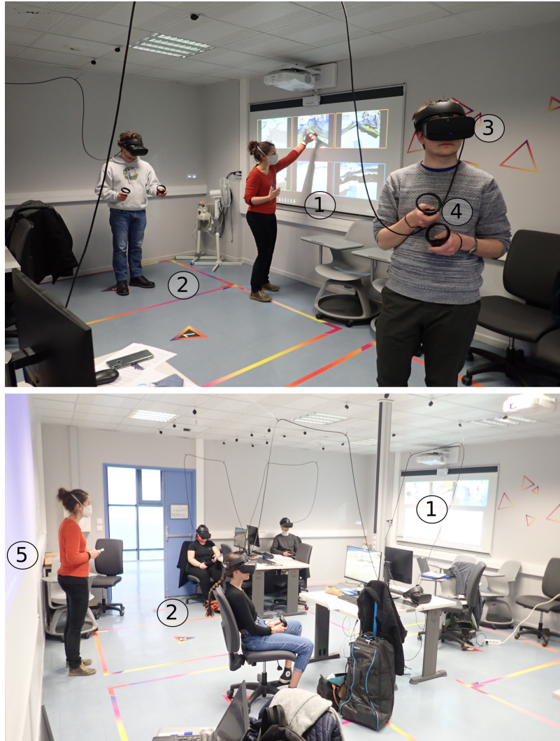
Figure 4. Views of virtual lab room in the “Alone in the field” or “single-user” mode in which teacher (in orange) is outside the virtual environment. 1- Solstice collaborative screen sharing system, 2- virtual box where limited real displacements of the user are allowed, 3- Oculus Rift S headset, 4- controllers, 5- projection screen for teacher computer. It is to note that some students prefer to operate in VR while seated, while others find it more natural to be standing or moving in the limit of their virtual box (2).
